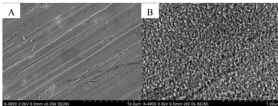
**Fig. S3** (A) Low and (B) high magnification SEM images of the copper foil in 20ml 0.2M  $\text{Na}_2\text{O}_2$  solution reacting for 6 hours without the addition of  $\text{AgNO}_3$ .
