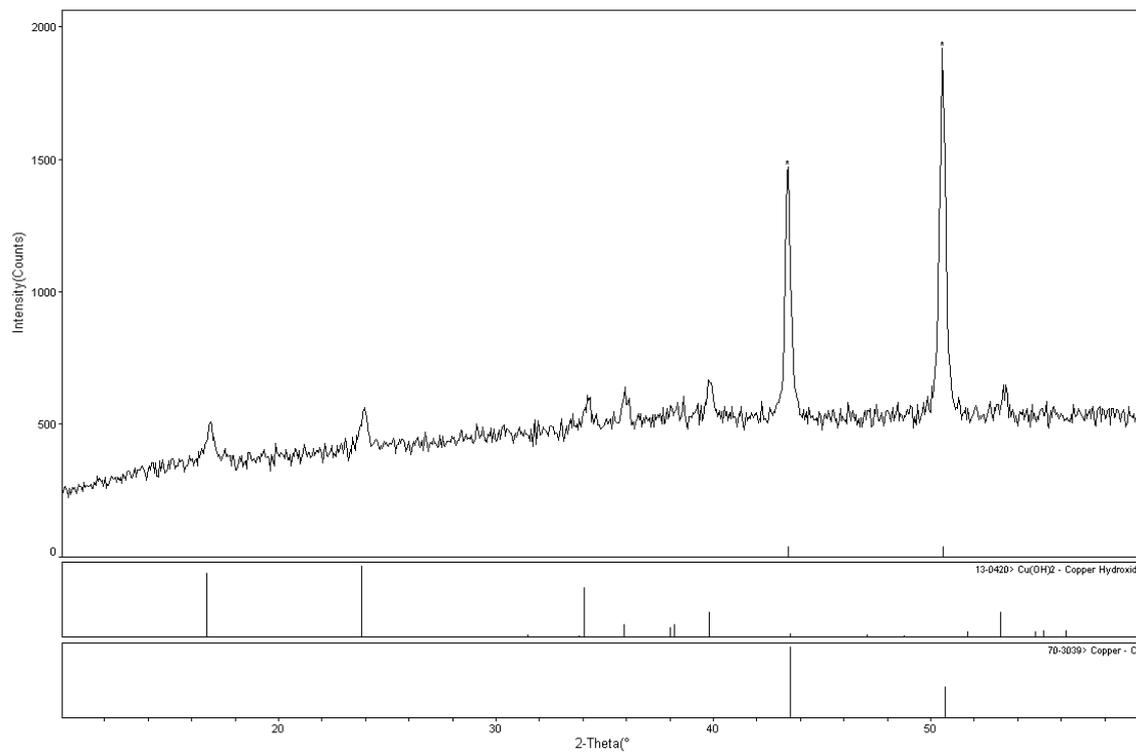
**Fig. S2** The XRD pattern of the  $\text{Cu}(\text{OH})_2$  nanoribbons modified copper foil at a scan rate of  $0.06^\circ/\text{sec}$  of  $2\theta$  range from  $10$  to  $70^\circ$ .
