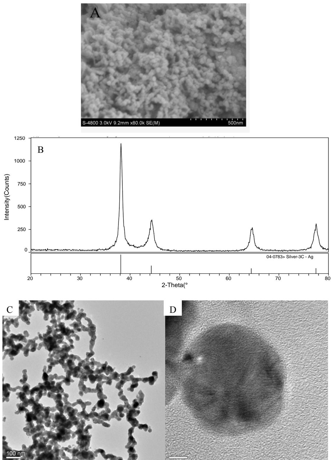
**Fig. S1** (A) SEM image. (B) XRD pattern of the as-prepared Ag nanoparticles at a scan rate of  $0.08^{\circ}/\text{sec}$  of  $2\theta$  range from  $20$  to  $80^{\circ}$ . (C) TEM and (D) HRTEM images of the Ag nanoparticles from a mixture solution containing  $0.2\text{M Na}_2\text{O}_2$  and  $3\text{mM AgNO}_3$ .
