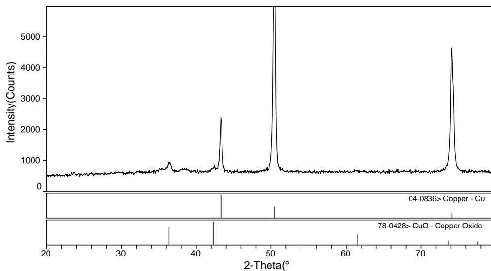
**Fig. S5** XRD of CuO nanoribbon array fabricated in the mixture solution containing 0.2M  $\text{Na}_2\text{O}_2$  and 3mM  $\text{AgNO}_3$  under ultrasonic irradiation at a scan rate of  $0.06^\circ/\text{sec}$  for  $2\theta$  range from 20 to  $80^\circ$ .
