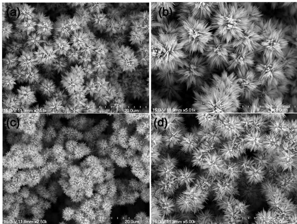
**FS2.** (a) and (b) FESEM images of ZnO multipods collected with copper sheet. (c) and (d) FESEM images of ZnO multipods collected with polyester film.
