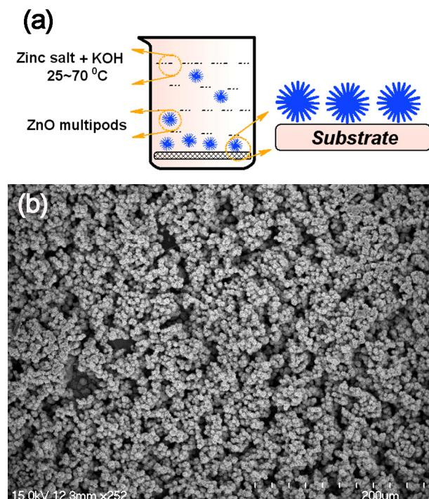
**FS1.** (a) Schematic description of the synthesis of ZnO multipods, where the substrate can be metal sheets, silicon wafer, glass, or flexible polyester film. (b) A low magnification FESEM image shows the extremely high yield of the multipods prepared via the above route.
