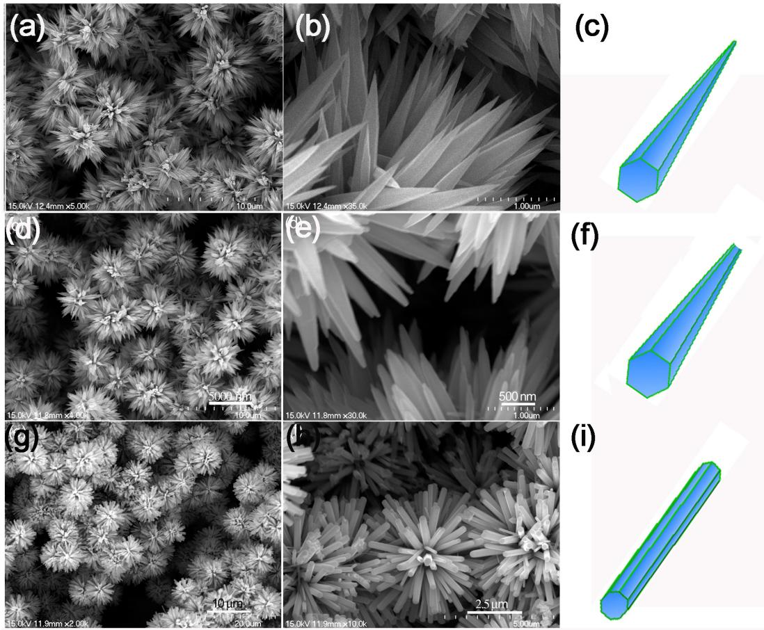
**FS3.** (a) and (b) FESEM images of ZnO multipods prepared at 25 °C. (c) Diagrammatic description of the shape of the branches of the multipods prepared at 25 °C. (d) and (e) FESEM images of ZnO multipods prepared at 50 °C. (f) Diagrammatic description of the shape of the branches of the multipods prepared at 50 °C. (g) and (h) FESEM images of ZnO multipods prepared at 70 °C. (i) Diagrammatic description of the shape of the branches of the multipods prepared at 70 °C.
