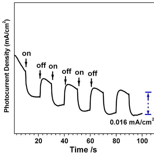
**FS6.** Short-circuit photocurrent density vs. time curves of  $\text{ZnO}/\text{Cu}_2\text{S}$  multipods. Electrolyte solution:  $0.1 \text{ mol/L Na}_2\text{SO}_4$ . Abnormally, the illumination of  $\text{ZnO}/\text{Cu}_2\text{S}$  multipods causes a dramatical decrease of the current, rather than the enhancement.
