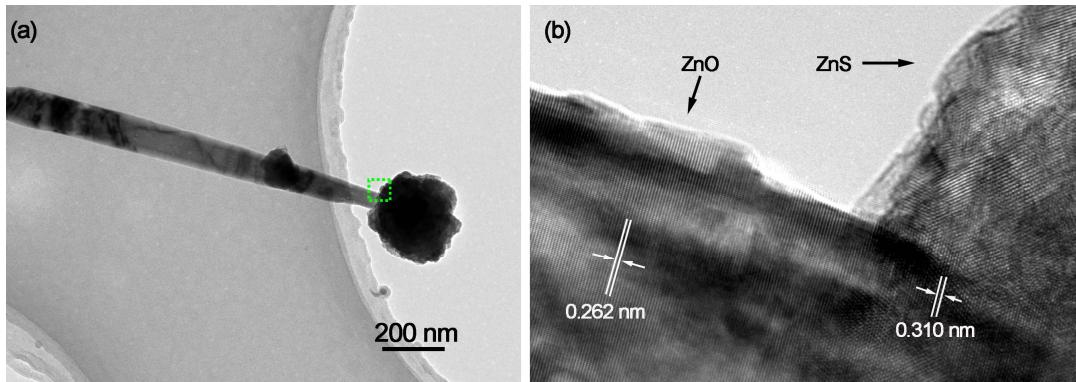
**FS4.** (a) TEM image shows the supporting of ZnS particle by the tip of the branch. (b) HRTEM image taken on the region marked by the box in Panel a, confirming that the polycrystalline ZnS particle is attached on ZnO.
