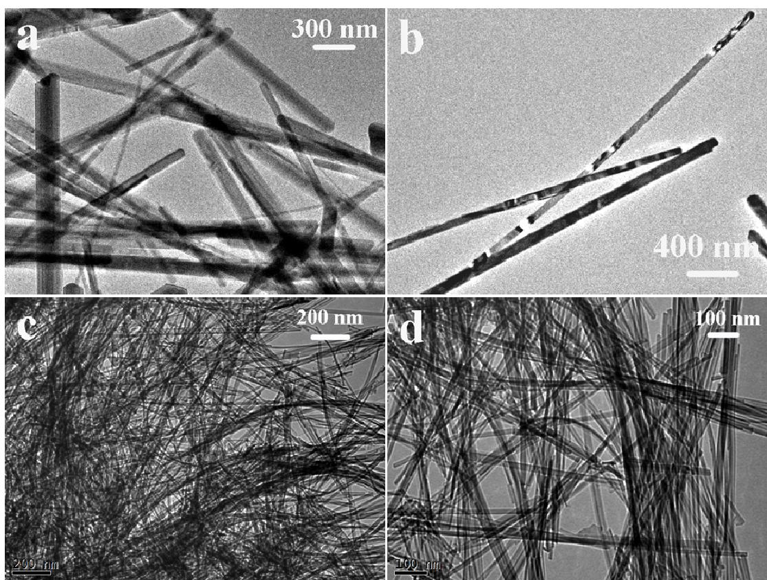
**Fig. SI2** TEM images of (a, b) MnOOH nanorods and (c, d) MnO<sub>2</sub> nanowires
