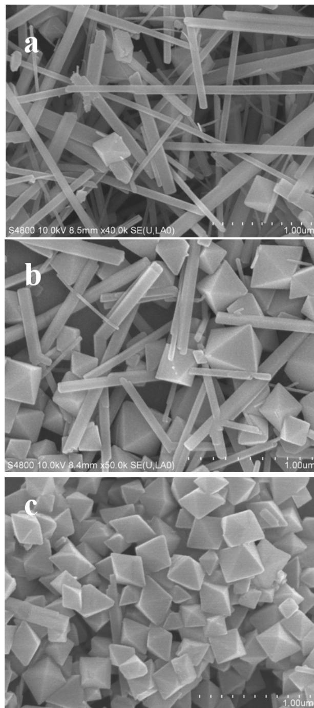
**Fig. SI4** SEM images of the products prepared with 0.1 g of KMnO<sub>4</sub> and (a) 5 mL of 10 g/L CMC solution; (b) 10 mL of 10 g/L CMC solution and (c) 20 mL of 20 g/L CMC solution under hydrothermal conditions at 140 °C for 6 h.
