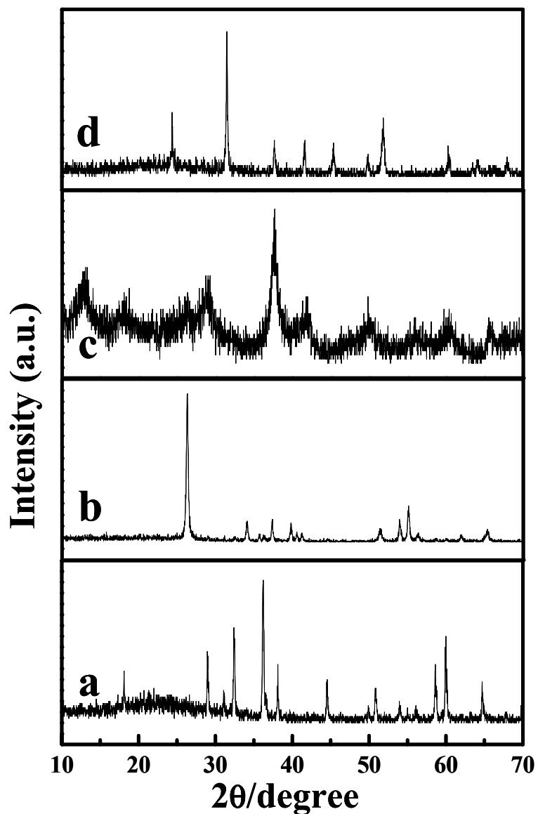
**Fig. SI1** XRD patterns of the obtained manganese-based nanostructures: (a) Mn<sub>3</sub>O<sub>4</sub> octahedrons; (b) MnOOH nanorods; (c) MnO<sub>2</sub> nanowires; (d) Aggregated MnCO<sub>3</sub> nanoparticles in the form of spindles.
