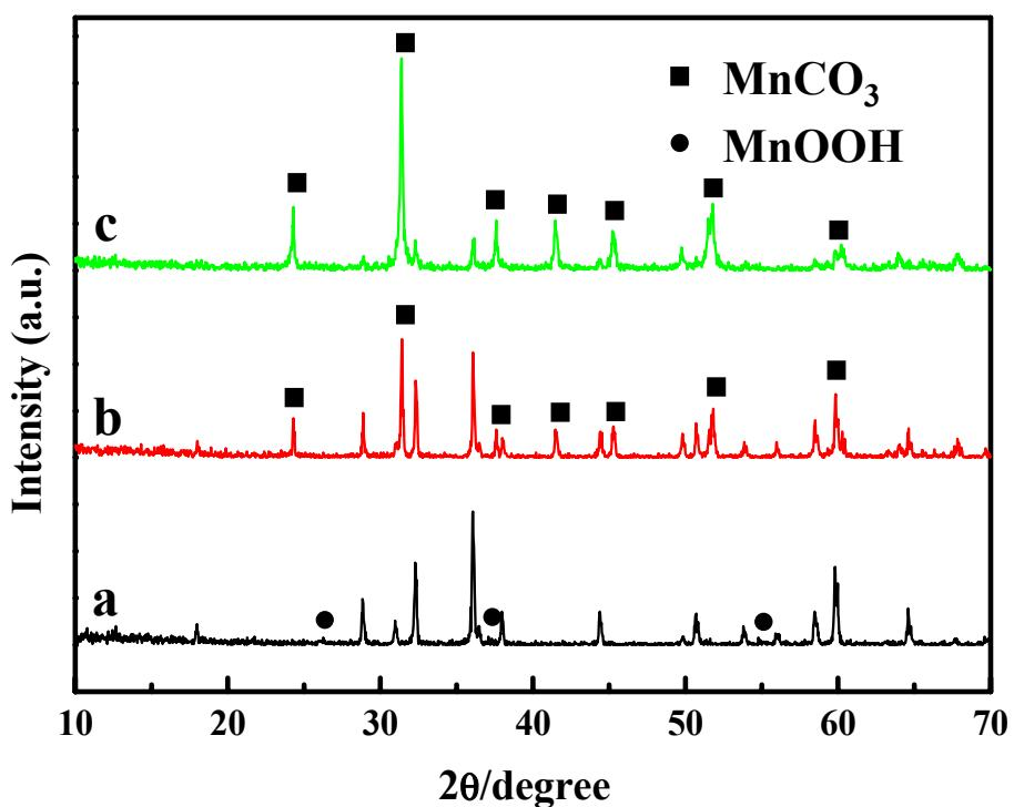
**Fig. SI5** XRD patterns of the products prepared with 0.1 g of  $\text{KMnO}_4$  and 20 mL of 10 g/L CMC solution under hydrothermal conditions for 6 h at (a) 120 °C, (b) 160 °C and (c) 200 °C. The diffraction peaks signed with “•” can be indexed as  $\text{MnOOH}$ , the diffraction peaks signed with “■” can be indexed as  $\text{MnCO}_3$  and the other diffraction peaks can be indexed as  $\text{Mn}_3\text{O}_4$ .
