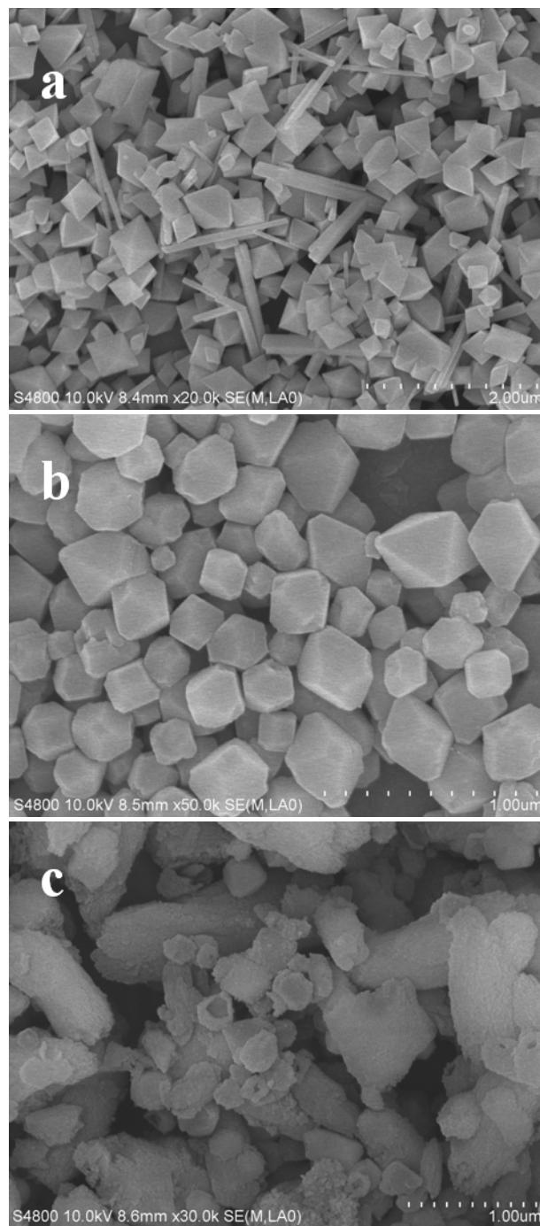
**Fig. SI6** SEM images of the products prepared with 0.1 g of KMnO<sub>4</sub> and 20 mL of 10 g/L CMC solution under hydrothermal conditions for 6 h at (a) 120 °C, (b) 160 °C and (c) 200 °C.
