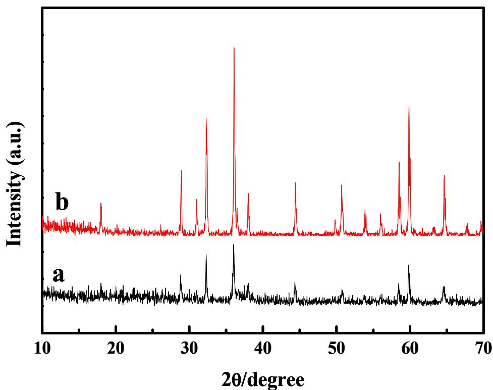
**Fig. SI7** XRD patterns of the products prepared with 0.1 g of KMnO<sub>4</sub> and 20 mL of 10 g/L CMC solution under hydrothermal conditions at 140 °C for (a) 2 h and (b) 4 h.
