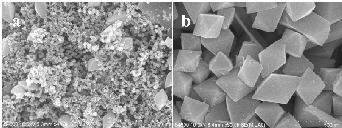
**Fig. SI8** SEM images of the products prepared with 0.1 g of KMnO<sub>4</sub> and 20 mL of 10 g/L CMC solution under hydrothermal conditions at 140 °C for (a) 2 h and (b) 4 h.
