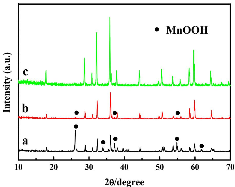
**Fig. SI3** XRD patterns of the products prepared with 0.1 g of KMnO<sub>4</sub> and (a) 5 mL of 10 g/L CMC solution; (b) 10 mL of 10 g/L CMC solution and (c) 20 mL of 20 g/L CMC solution under hydrothermal conditions at 140 °C for 6 h. The diffraction peaks signed with “●” can be indexed as MnOOH and the other diffraction peaks can be indexed as Mn<sub>3</sub>O<sub>4</sub>.
