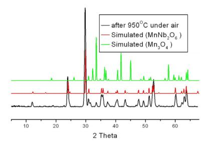
Figure S2. Comparison of powder patterns of 1 after 950°C with that simulated from  $MnNb_2O_6$  and  $Mn_3O_4$ .
