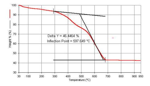
Figure S1. TGA plot heated from 30 °C to 950 °C at 5 °C /min under a flow of air (40 mL/min).
