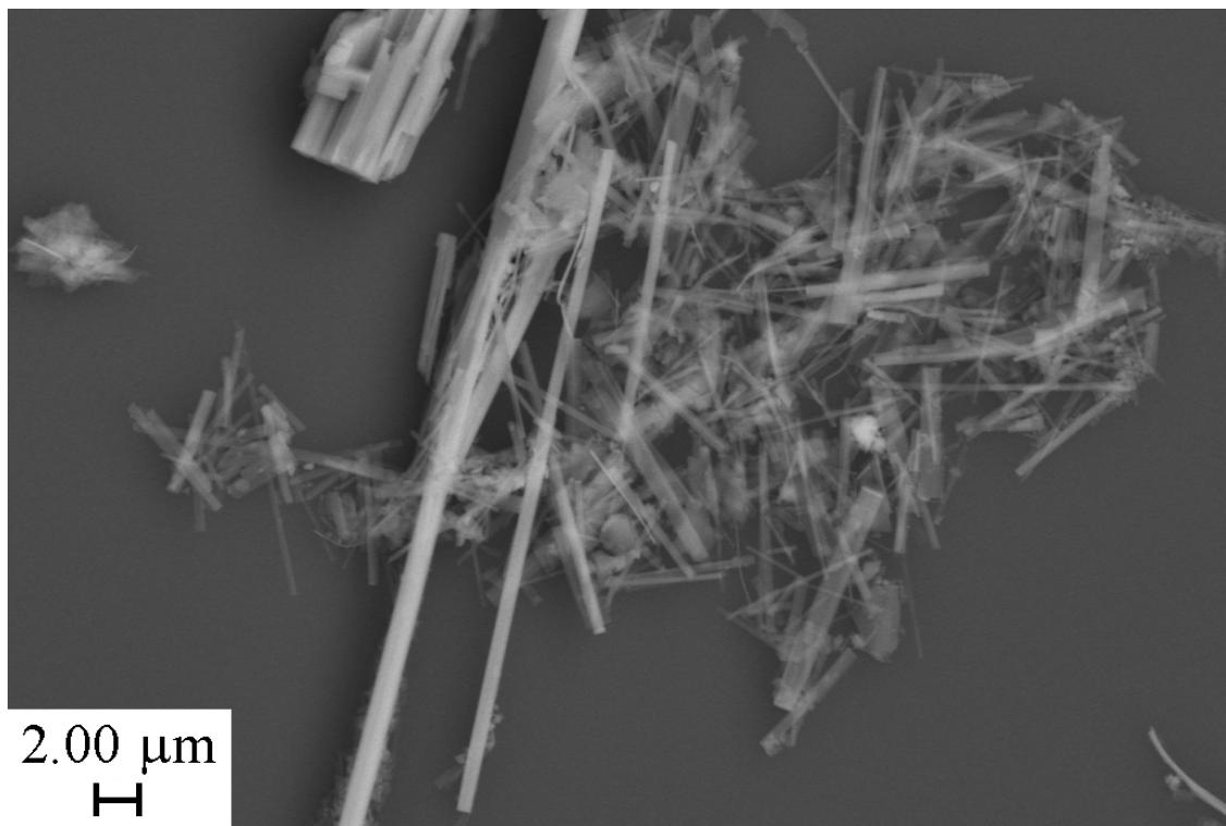
**Figure S1.** SEM image of as-prepared  $\text{Nb}_2\text{O}_5$  nanowires.
