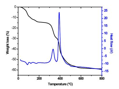
Figure S1: TG and DTG curves of  $Eu_2(H_2O)_4$  (pzdc)<sub>3</sub>  $3H_2O$  (4) under air (heating rate:  $1^{\circ}C.min^{-1}$ ).
