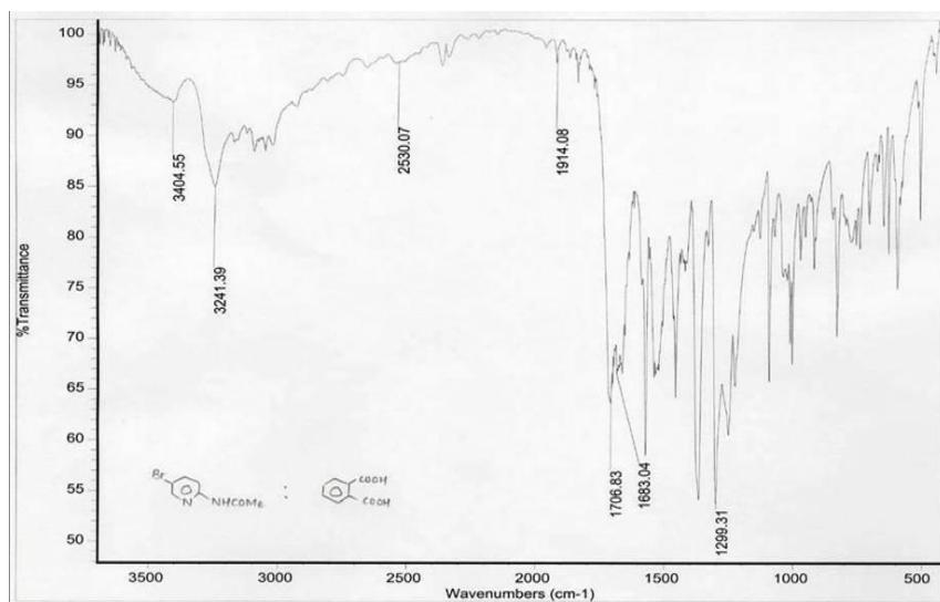
IR spectrum of the attempted co-crystallization of 2-acetamido-5-bromopyridine & pthalic acid, **f12** (no reaction).
