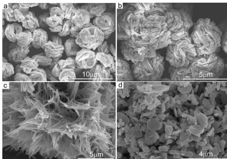
**Fig. S1.** SEM images of the products obtained at 80°C for 24h without any additives (a) and with different additives (b) CPC, (c) SDS, (d) P123.
