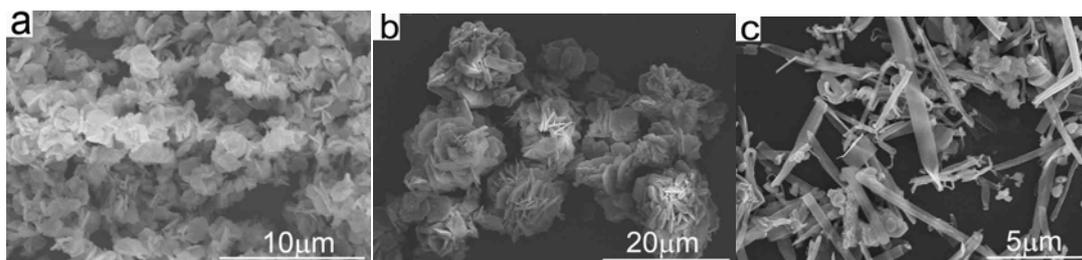
**Fig. S3.** SEM image of the products obtained under different reaction temperature: (a) 50 °C, (b) 160 °C, and (c) 180 °C.
