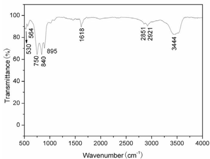
**Fig. S4.** FT-IR spectrum of the as-prepared  $\text{Cu}_3\text{V}_2\text{O}_7(\text{OH})_2 \cdot 2\text{H}_2\text{O}$  samples.
