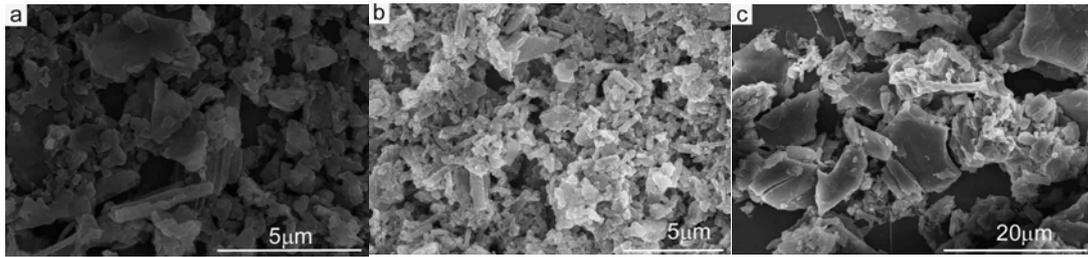
**Fig. S2.** SEM images of the samples prepared from the system with different copper sources : (a)  $\text{CuSO}_4 \cdot 5\text{H}_2\text{O}$ , (b)  $\text{CuCl}_2 \cdot 2\text{H}_2\text{O}$ , and (c)  $\text{Cu}(\text{NO}_3)_2 \cdot 5\text{H}_2\text{O}$ .
