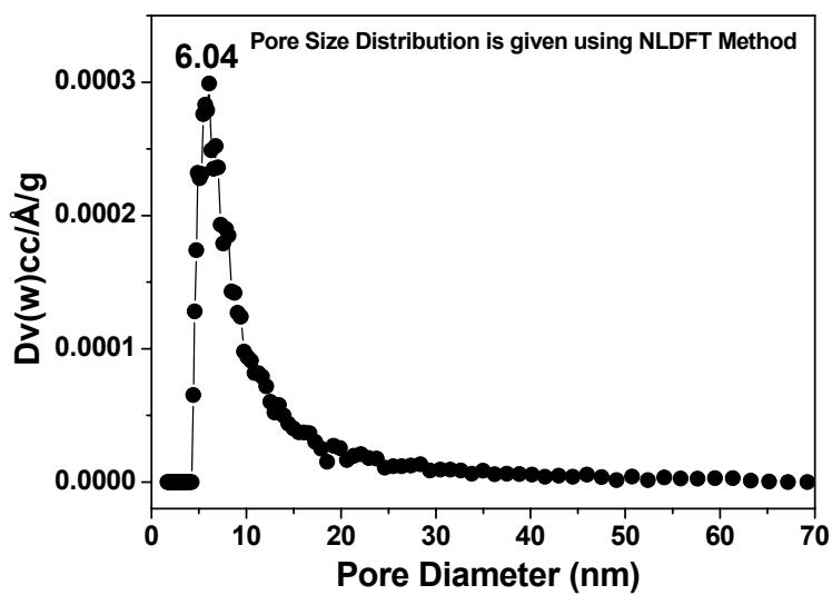
ESI Figure S4: The pore size distribution curve of tri-peptide **1** exhibits a peak at 6.04 nm indicating the mesoporous architecture.
