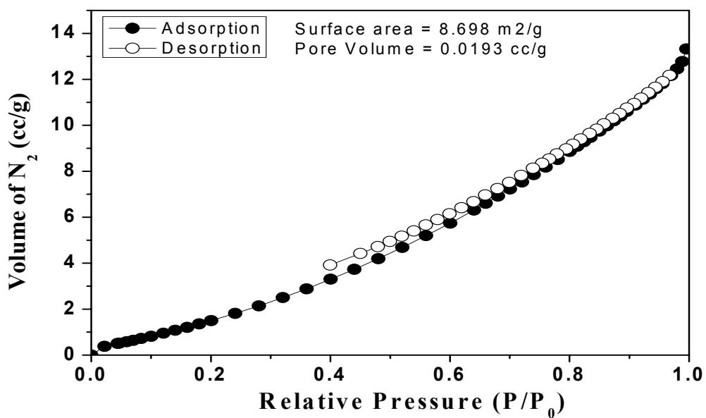
ESI Figure S3: The N<sub>2</sub> gas adsorption /desorption isotherms (77K) of tri-peptide **1** is close to the type 1 adsorption isotherm typical for a nanoporous material.
