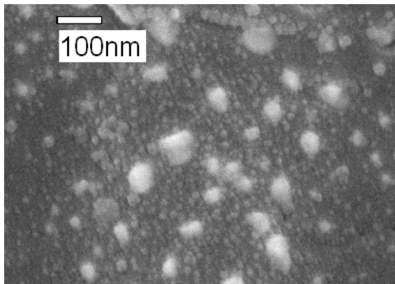
Figure S6. The formation of GNP with different size and shape from a tripeptide Boc-Phe-Phe-Tyr-OMe, which does not exhibits nanoporous structure.
