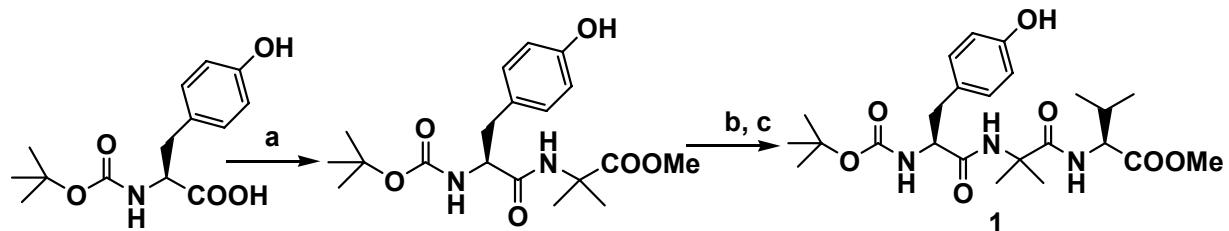
ESI Figure S1: Schematic presentation of synthesis of tripeptide **1**. Reagents and conditions: (a) DMF, H-Aib-OMe, DCC, HOEt, 0°C, 90% yield; (b) MeOH, 2M NaOH, 85% yield; (c) DMF, H-Val-OMe, DCC, HOEt, 0°C, 80% yield.
