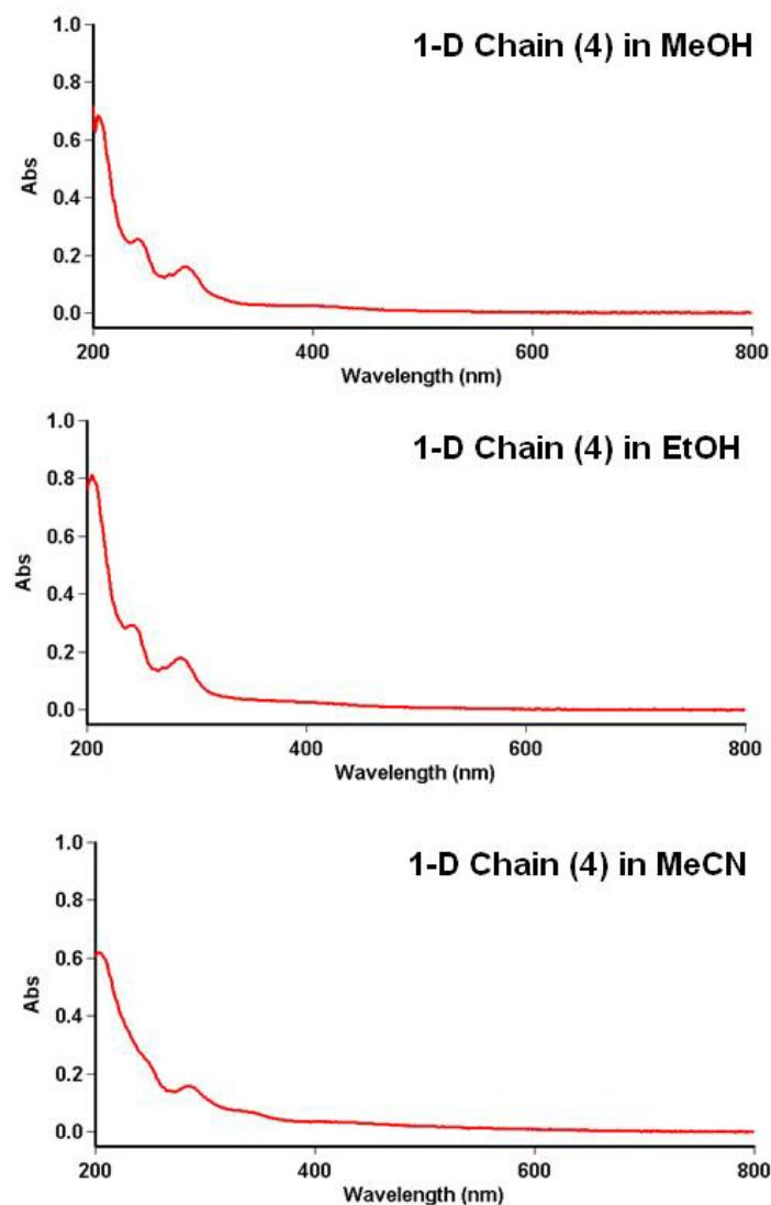
**Fig. SI8** UV/vis spectra obtained from MeOH (top), EtOH (middle) and MeCN (bottom) solutions of the 1-D chain in **4**.
