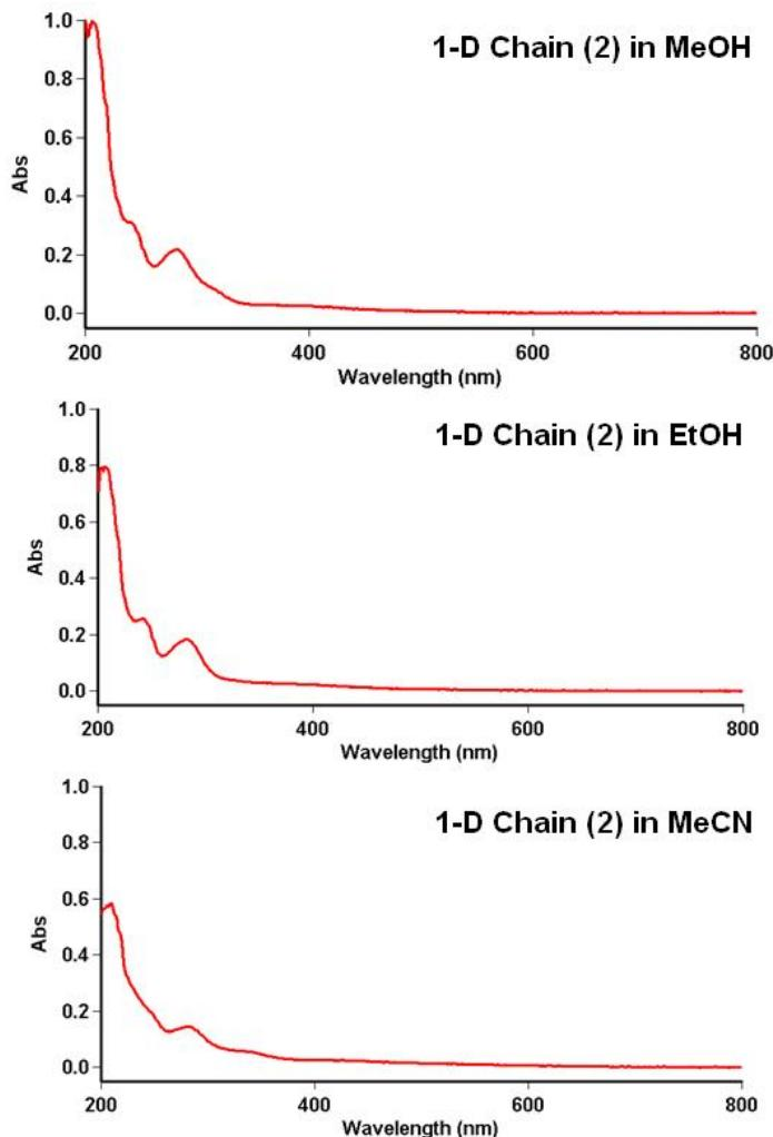
**Fig. SI7** UV/vis spectra obtained from MeOH (top), EtOH (middle) and MeCN (bottom) solutions of the 1-D chain in **2**.
