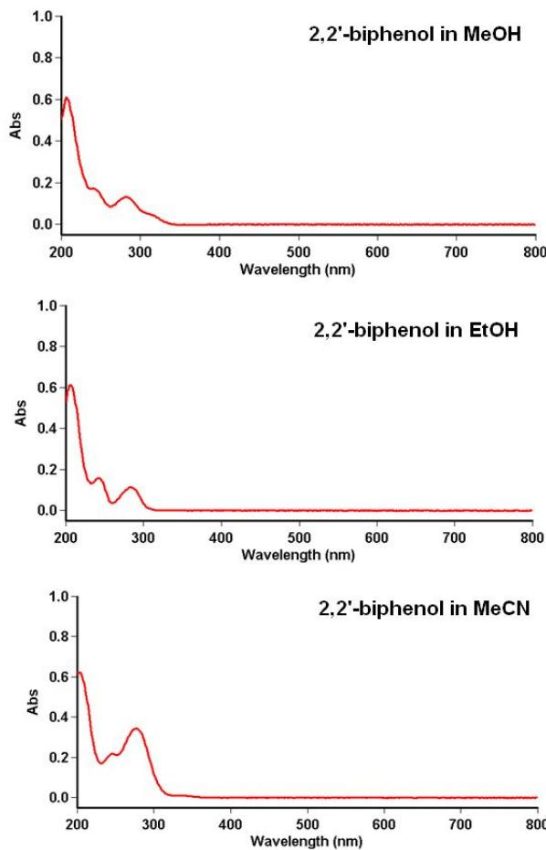
**Fig. SI6** UV/vis spectra obtained from MeOH (top), EtOH (middle) and MeCN (bottom) solutions of 2,2'-biphenol. UV/vis (MeOH):  $\lambda_{\text{max}}$  [nm] ( $\epsilon_{\text{max}} \text{ } 10^3 \text{ dm}^3 \text{ mol}^{-1} \text{ cm}^{-1}$ ): 206 (37.9), 241 (10.8), 292 (8.2), 318(sh). (EtOH): 207 (38.1), 243 (9.8), 284 (8.3). (MeCN): 203 (38.6), 246 (13.6), 277 (21.2), 319 (2.6).
