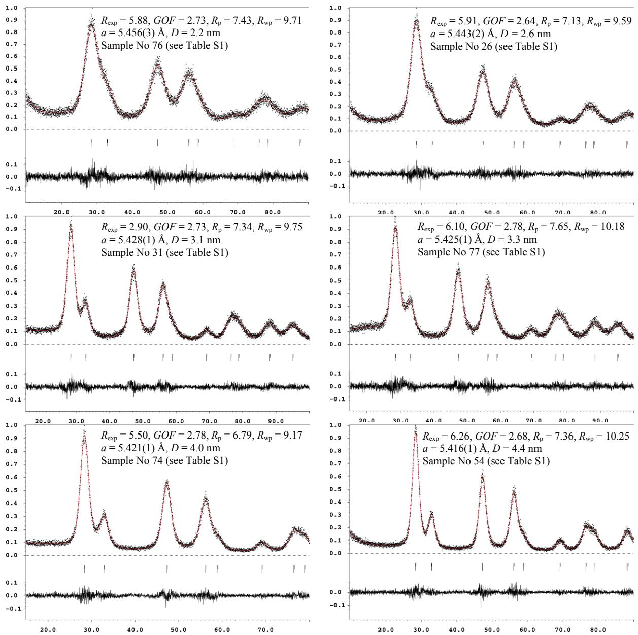
**Figure S1.** Rietveld refinement of selected ceria samples (particle size 2.2–23.5 nm).
