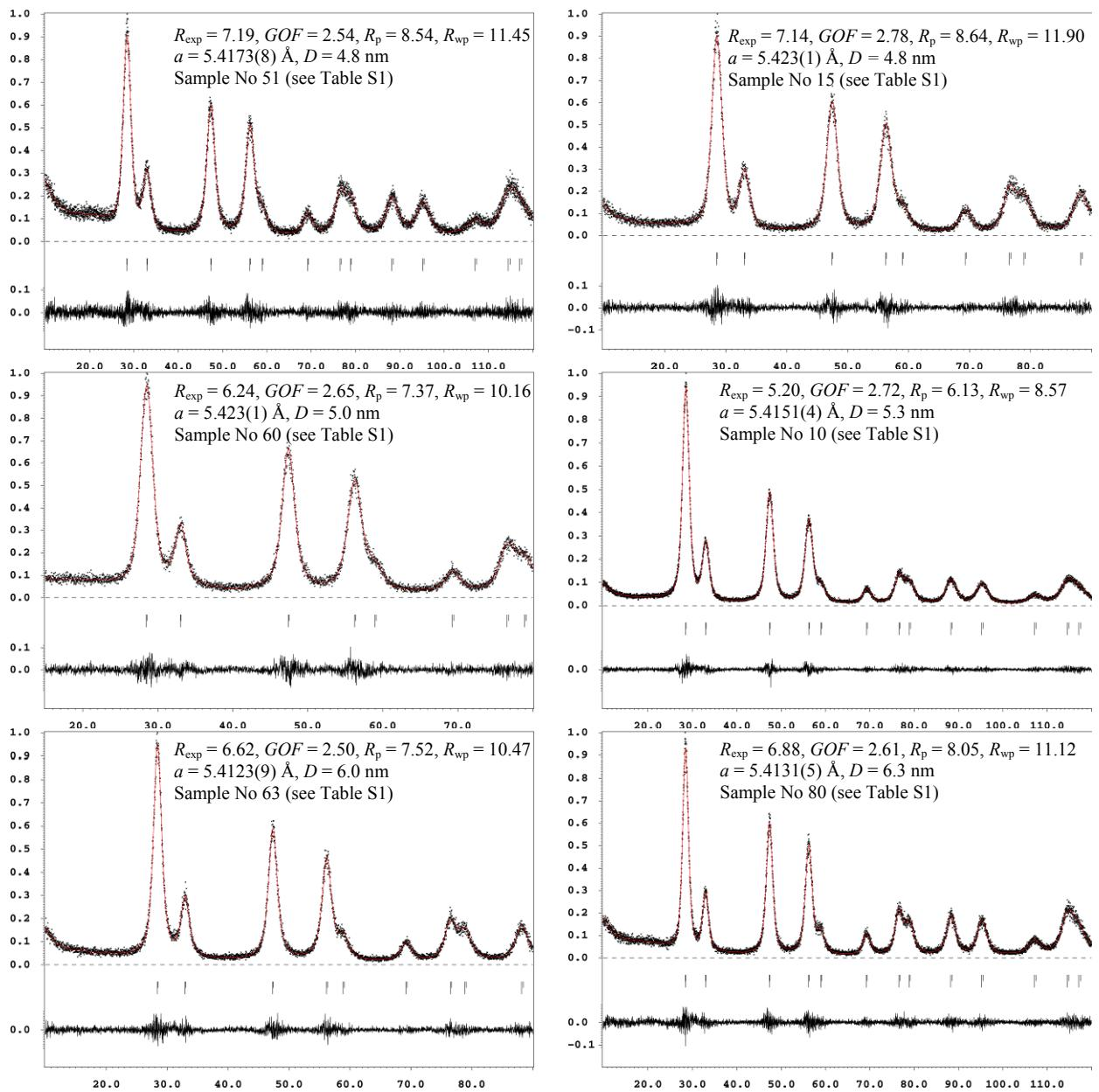
**Figure S1 (contd.). Rietveld refinement of selected ceria samples (particle size 2.2–23.5 nm).**
