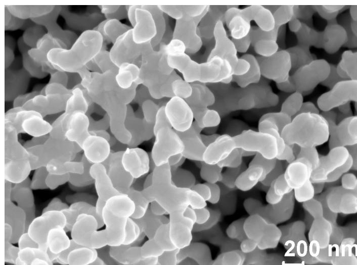
**Fig. E3 SEM micrograph showing the microstructure of nanoporous Ag by dealloying the melt-spun Mg<sub>65</sub>Ag<sub>35</sub> alloy in the 5 wt.% HCl aqueous solution.**
