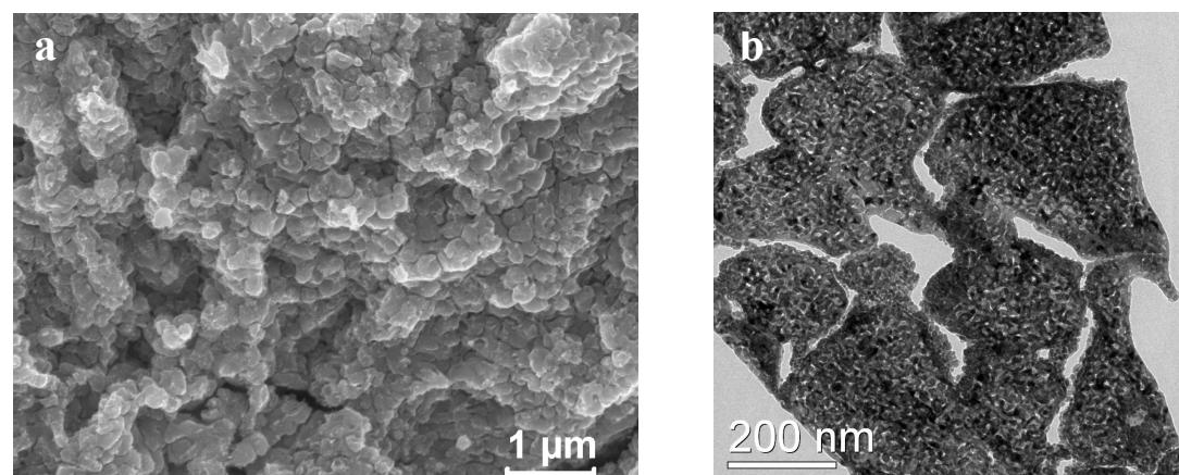
**Fig. E1 (a)** SEM and **(b)** TEM micrographs showing the microstructure of the nanoporous Ag<sub>80</sub>Pd<sub>20</sub> alloy by dealloying the rapidly solidified Mg<sub>60</sub>Ag<sub>32</sub>Pd<sub>8</sub> alloy in the 5 wt.% HCl aqueous solution.
