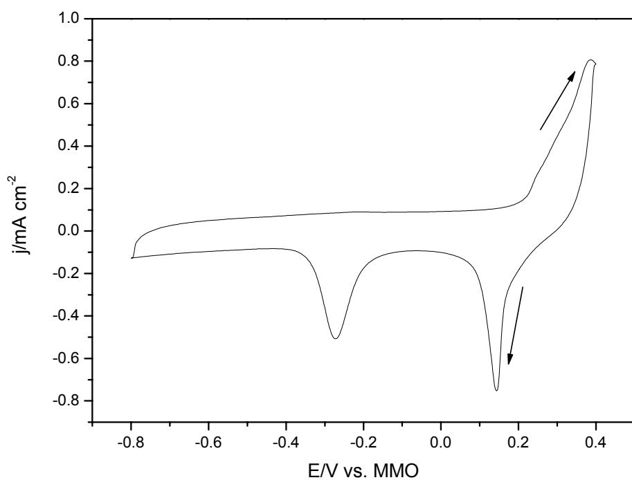
**Fig. E5** CV for the nanoporous  $\text{Ag}_{80}\text{Pd}_{20}$  electrode in the 1 M KOH solution. Scan rate:  $50 \text{ mV s}^{-1}$ .
