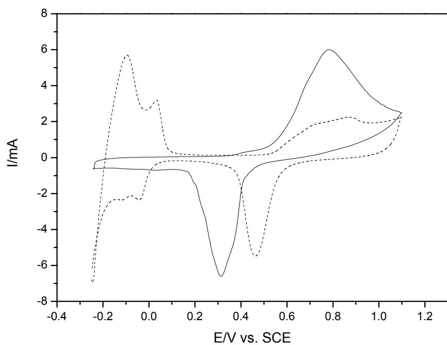
Fig. E4 CVs for the nanoporous  $\text{Ag}_{80}\text{Pd}_{20}$  electrode (solid line) and the nanoporous Pd electrode (dash line) in the 1M  $\text{H}_2\text{SO}_4$  solution. Scan rate: 50 mV s<sup>-1</sup>.
