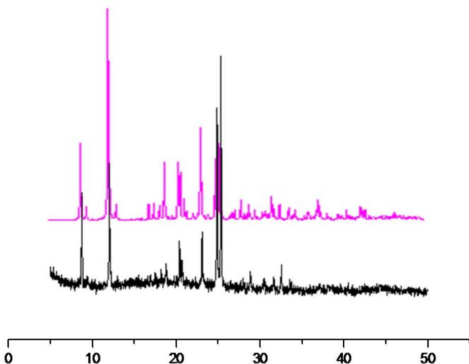
Fig. S6 The simulated X-ray powder diffraction patterns (upper) and the measured one (lower) of complex **3**
