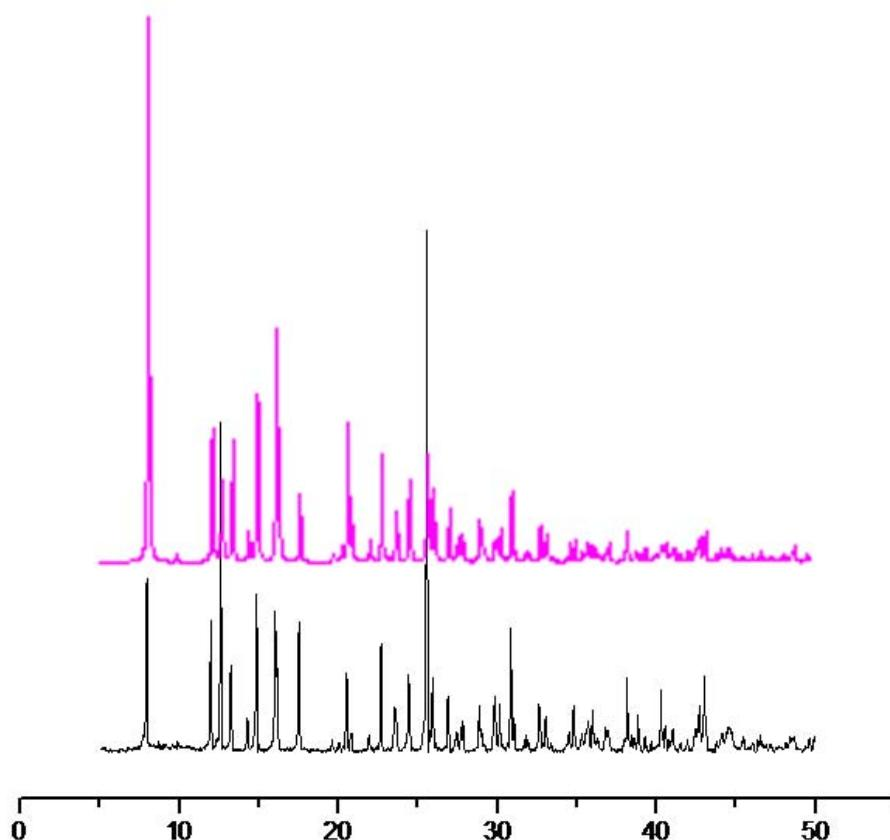
Fig. S4 The simulated X-ray powder diffraction patterns (upper) and the measured one (lower) of complex **1**
