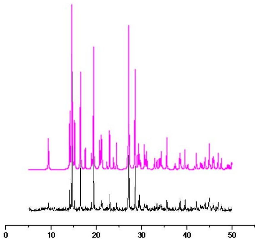
Fig. S5 The simulated X-ray powder diffraction patterns (upper) and the measured one (lower) of complex **2**
