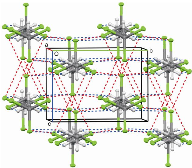
**Fig. S1.** The crystal structure of 111TCE at 2.15 GPa/295 K. The dashed red and blue lines indicate the shortest Cl···Cl and Cl···H intermolecular distances, respectively (Table S3). Displacement ellipsoids are plotted at the 25% probability level.
