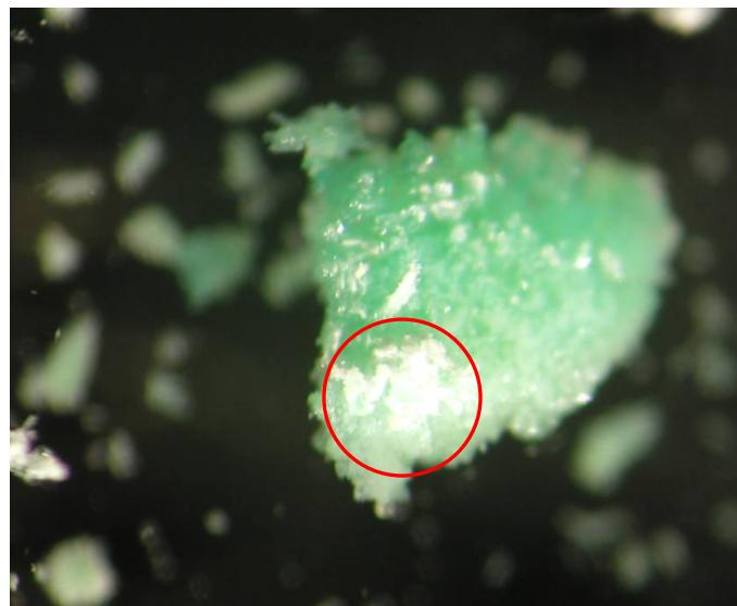
Figure S2. Dimerization reaction in *p*-bromonitrosobenzene after 15 minutes. Circled part of the sample which turned white is exposed to air while the rest of the sample is immersed in glycerol.
