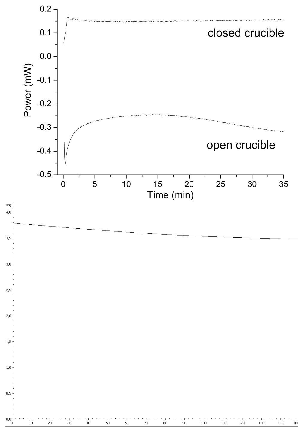
Figure S4. (top) Isothermal DSC thermograms of samples of solid *p*-bromonitrosobenzene undergoing dimerisation in a closed (top) and in an open (bottom) crucible. Exo is up. The crucibles were maintained at constant temperature of 30 °C. (bottom) Isothermal mass measurement during dimerisation of *p*-bromonitrosobenzene.
