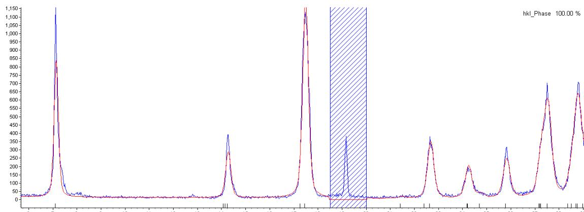
Figure S9. Le Bail fit of the final dimerization product using the unit cell of the dimer of *p*-bromonitrosobenzene. Shaded region is excluded due to an unidentified impurity; this peak did not change in time during the dimerization.
