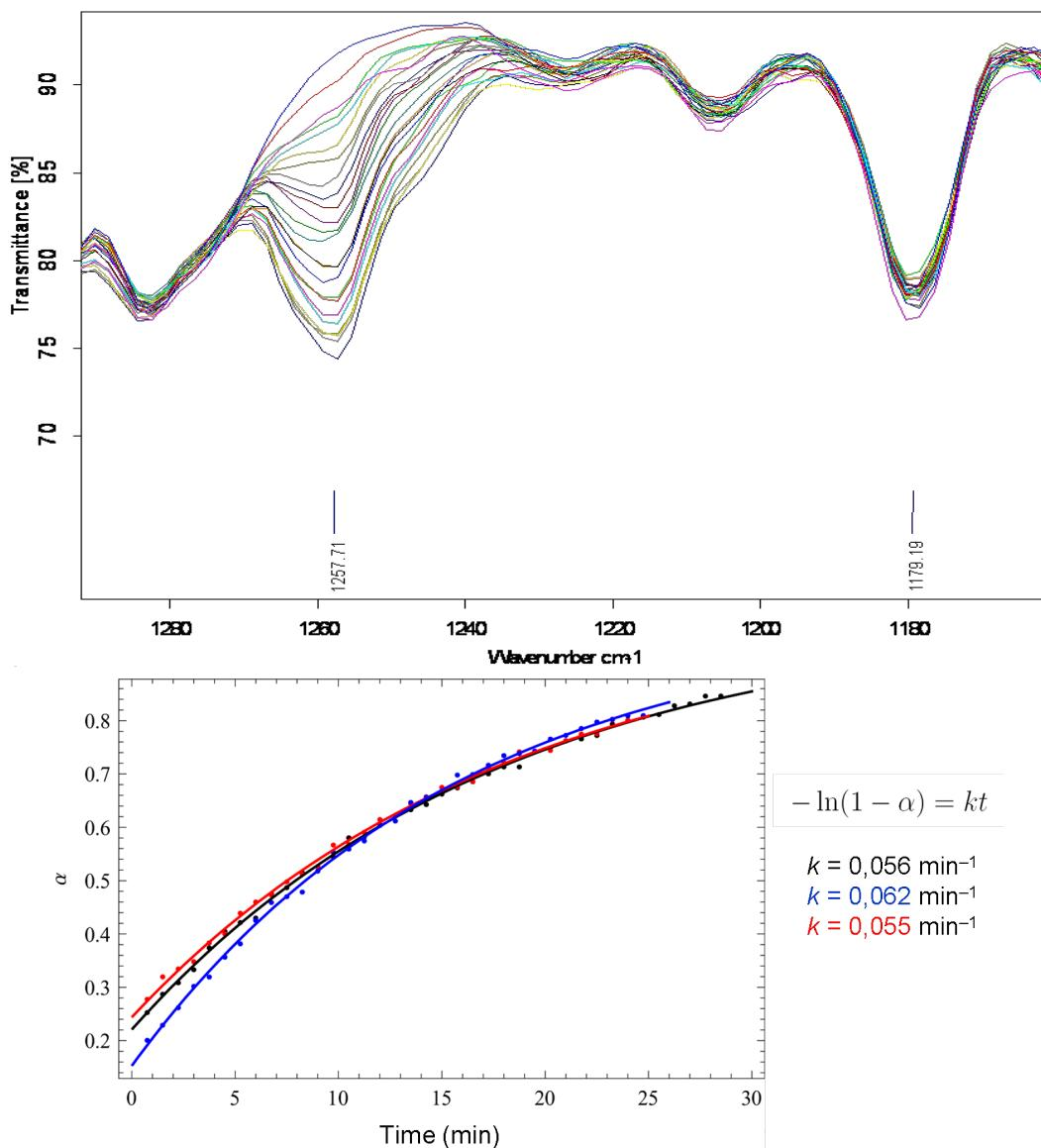
Figure S10. (top) Time-resolved IR spectra of *p*-bromonitrosobenzene. The band at 1258 cm<sup>-1</sup> belonging to the asymmetric stretching of the ONNO group of the dimer is increasing in intensity. (bottom) Fitting the reaction rate law of the first order to the intensity change of the ONNO stretching of *p*-bromonitrosobenzene from time resolved infrared spectra. Three independent data sets.
