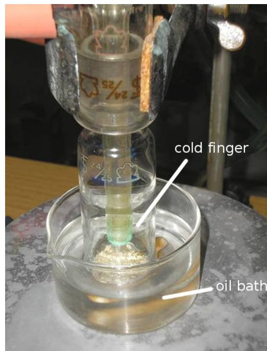
Figure S3. Sublimation apparatus. A green monomer is formed on the cold finger.
