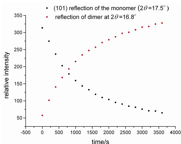
Figure S8. Change in selected reflection intensities of the monomer and of the dimer during dimerization of *p*-nitronitrosobenzene.
