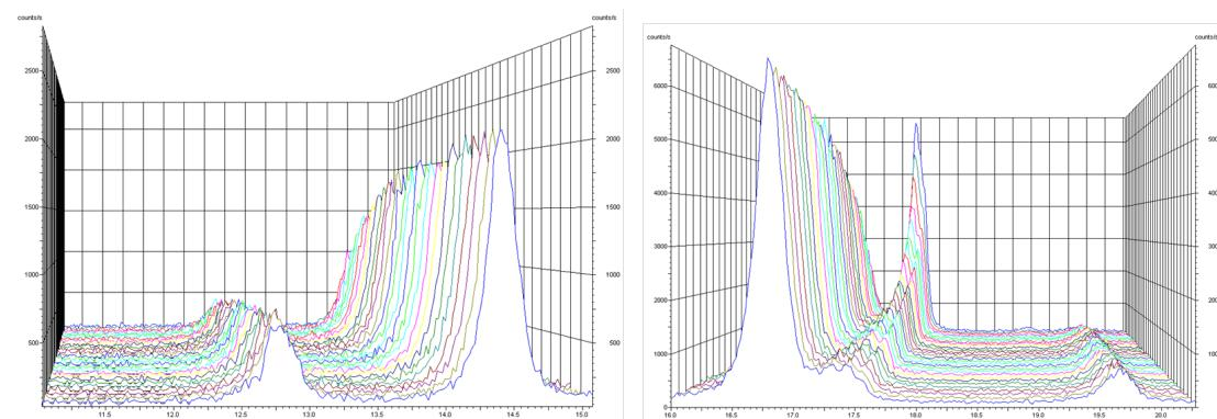
Figure S5. Solid-state dimerization of the *p*-nitronitrosobenzene measured by time-resolved powder X-ray diffraction. The first pattern is in the back, the last in the front. Patterns are separated 3 minutes and 20 seconds in time. (left)  $2\theta$  from  $11^\circ$  to  $15^\circ$  and (right) from  $15^\circ$  to  $21^\circ$ .
