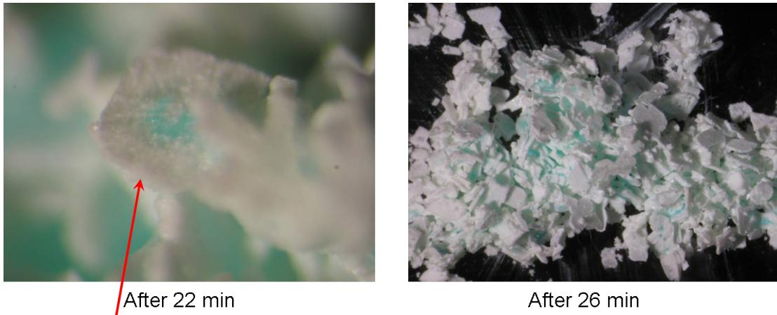
Figure S1. Solid-state dimerization of *p*-chloronitrosobenzene. (left) The arrow indicates crystal growth of the dimer phase which extends to the middle of the surface after having started at crystal edges. (right) In the bunch of crystals, those which are closer to edges of the bunch turn white sooner than those which are in the middle of the bunch. This is probably caused by higher vapour pressure inside the bunch of crystals and thus slower molecule loss by sublimation.
