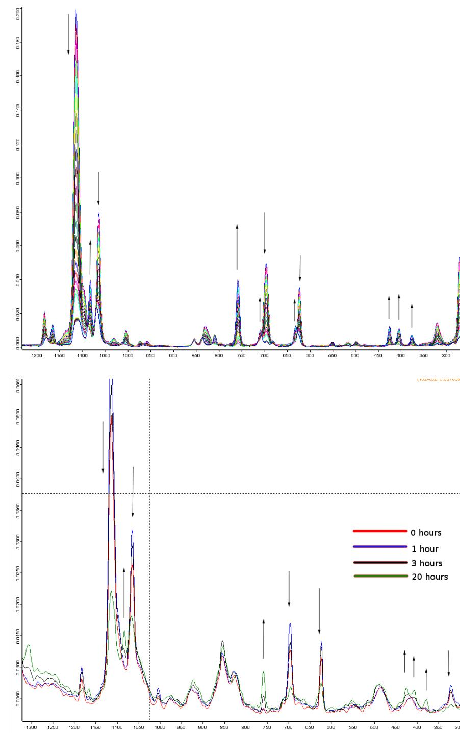
Figure S11. Time resolved Raman spectra of (top) an open sample of *p*-bromonitrosobenzene and (bottom) the sample immersed in glycerol. Spectra of the open sample are separated by three minutes in time. Formation of the dimer is best observable with the line at 758 cm<sup>-1</sup> since it is not overlapping with monomer bands or with glycerol. Arrows indicate whether the band is increasing or decreasing in intensity.
