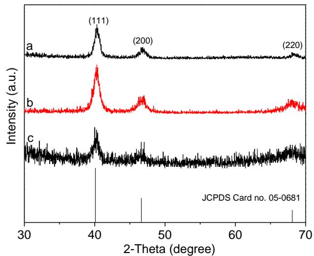
**Figure S1:** XRD patterns of (a) urchin-like, (b) flower-like and (c) pompon-like Pd particles prepared with 0.5 mM  $\text{H}_2\text{PdCl}_4$ .
