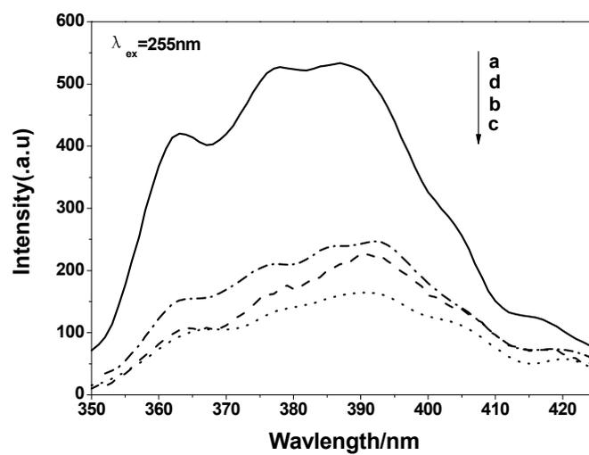
**Fig. S13** PL spectra of BiOCl hollow microspheres (a) and iodine-containing BiOCl with (b) hollow, (c) shell-core, and (d) solid structure.
