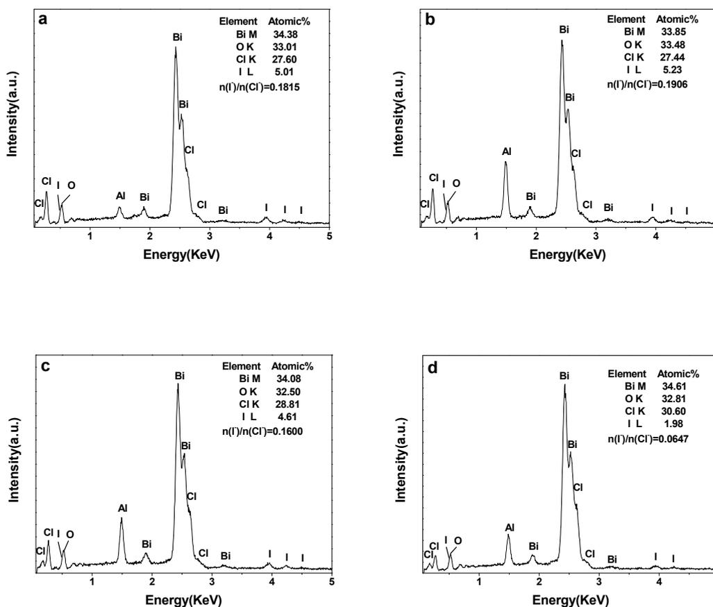
**Fig. S1** EDS analysis of iodine-containing BiOCl core-shell microsphere produced in 1.350 mmol NaI solution at 80 °C for different times: (a) 30 sec, (b) 1 min, (c) 4 min, and (d) 3 hours.
