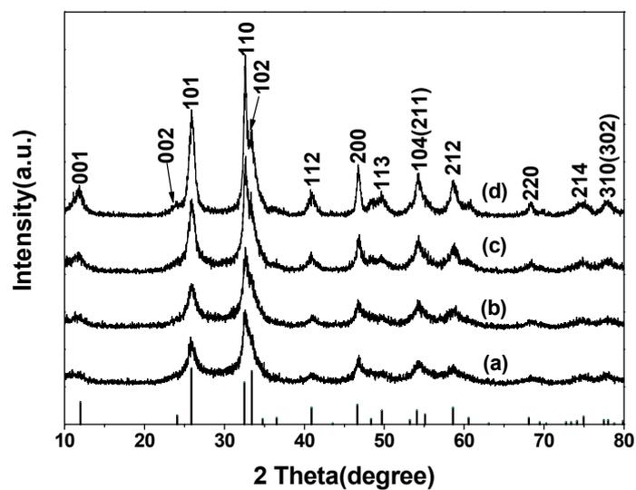
**Fig. S3** XRD patterns of pure BiOCl products without iodine-incorporation harvested at different intervals of reaction times: (a)30s, (b)1min, (c)4min and (d)3hours (Inset the standard card: JCPDS 06-0249).
