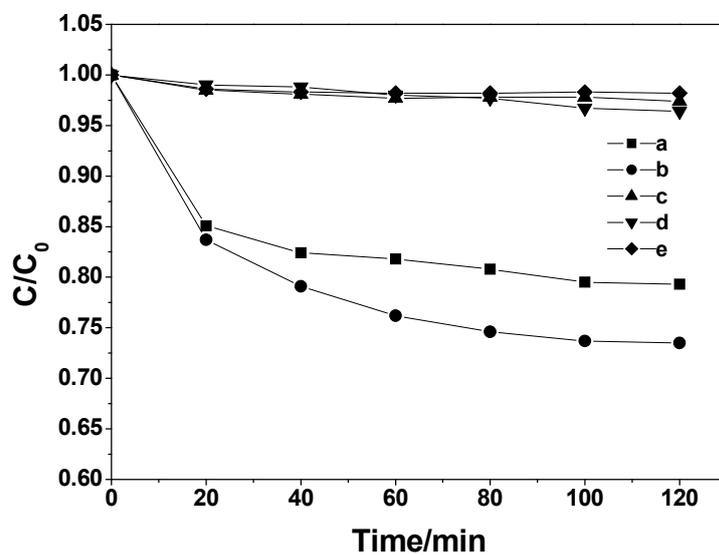
**Fig. S7** Comparison of the adsorption-desorption equilibrium of iodine-incorporated BiOCl (I-BiOCl) with (a) hollow, (b) core-shell, (c) solid structure, (d)  $\text{TiO}_{2-x-y}\text{N}_x\text{F}_y(\text{SC})-3$  with (e)  $\text{Bi}_2\text{WO}_6$ .
