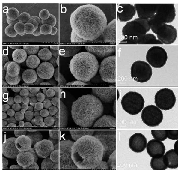
**Fig. S2** FESEM and TEM images of pure BiOCl products without iodine-incorporation harvested at different intervals of reaction times, (a-c) 30 sec, (d-f) 1 min, (g-i) 4min, (j-l) 3hours.
