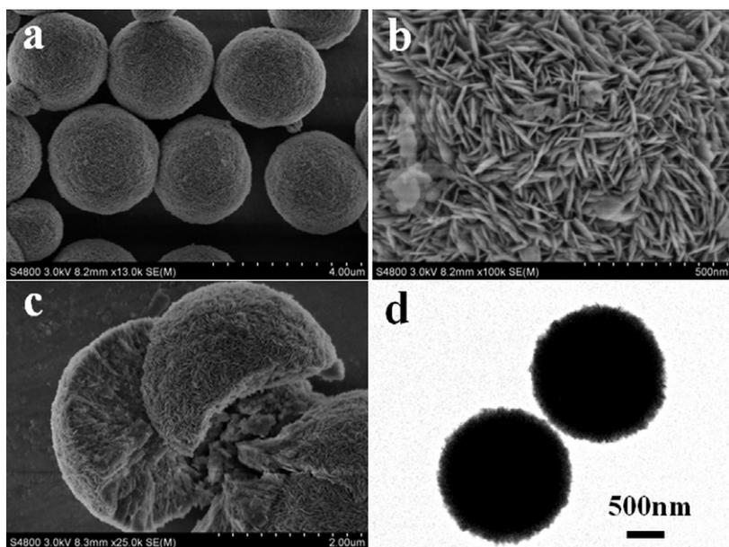
Fig. S5 (a-c) FESEM images of iodine-incorporation BiOCl (I-BiOCl) powders obtained without using PVP, (d) TEM images of iodine-incorporation BiOCl (I-BiOCl) powders.
