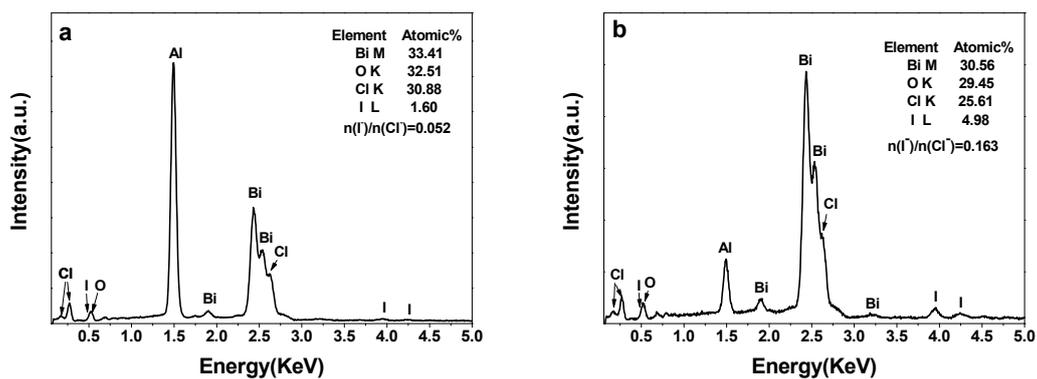
Fig. S4 EDS analysis on the atomic percentages of the iodine-incorporated (a) hollow and (b) solid BiOCl samples.
