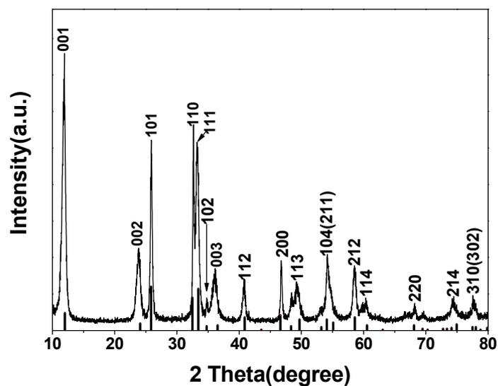
**Fig. S6** XRD of iodine-incorporation BiOCl (I-BiOCl) powders obtained without using PVP.
