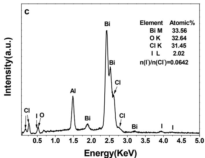
**Fig. S11** (a) XPS survey spectrum of iodine-incorporated BiOCl core-shell sample before and after irradiation, (b) high-resolution XPS spectra of the I3d region taken on the iodine-incorporated BiOCl core-shell sample before and after irradiation, (c) EDS analysis on the atomic percentages of the iodine-incorporated core-shell sample after irradiation.
