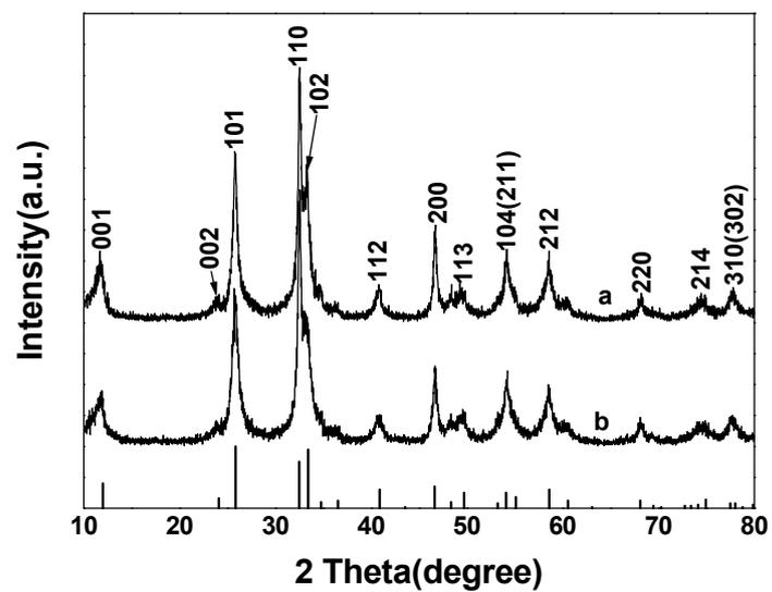
**Fig. S9** XRD pattern of the iodine-incorporated core-shell BiOCl sample (a) before and (b) after the photocatalytic reaction. (Inset the standard card: JCPDS 06-0249)
