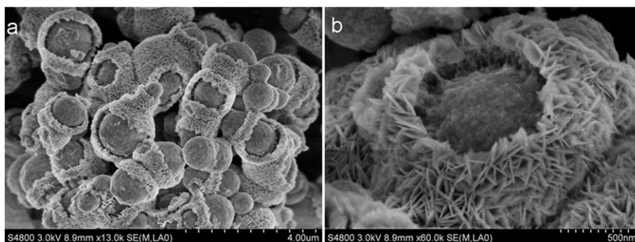
**Fig. S10** FESEM images of the iodine-incorporated BiOCl core-shell sample after the photocatalytic reaction.
