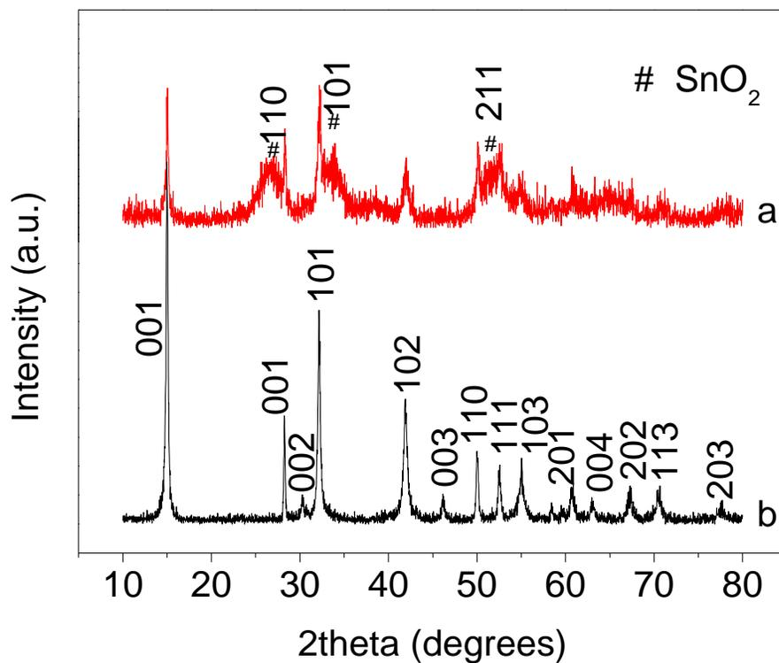
**Figure S4** XRD patterns of the samples synthesized under the same condition except with at different temperature: (a) 150 °C and (b) 210 °C.
