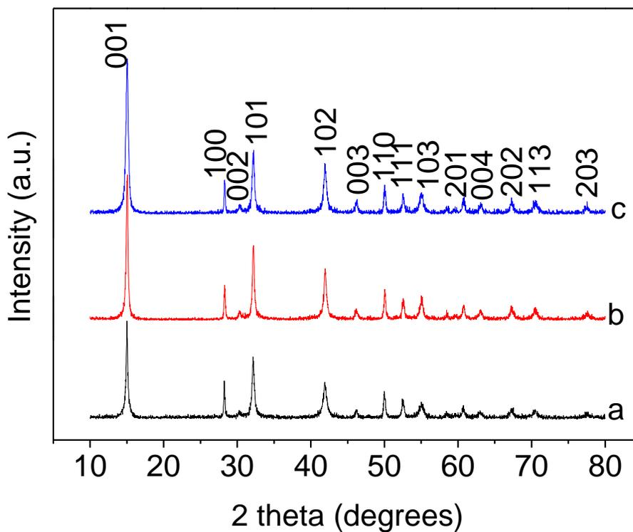
**Figure S2** XRD patterns of the samples synthesized under the same condition except with different amount of Tu: (a) 0.3 g; (b) 0.6 g and (c) 0.8 g.
