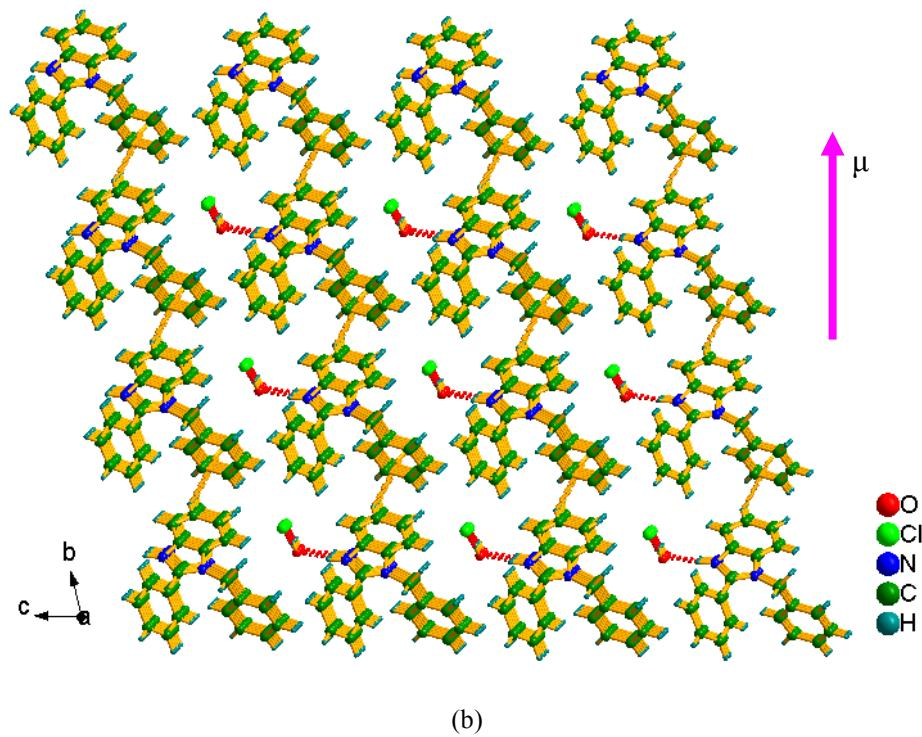
**Fig. S6** (a) 2D supramolecular layer in **3** along the  $c$  axis. (b) Packing diagram of **3** along the  $a$  axis. The red dashed-lines and yellow ones stand for hydrogen bonding and C-H $\cdots\pi$  packing interactions, respectively. The purple arrow denotes the direction of packing polarity.
