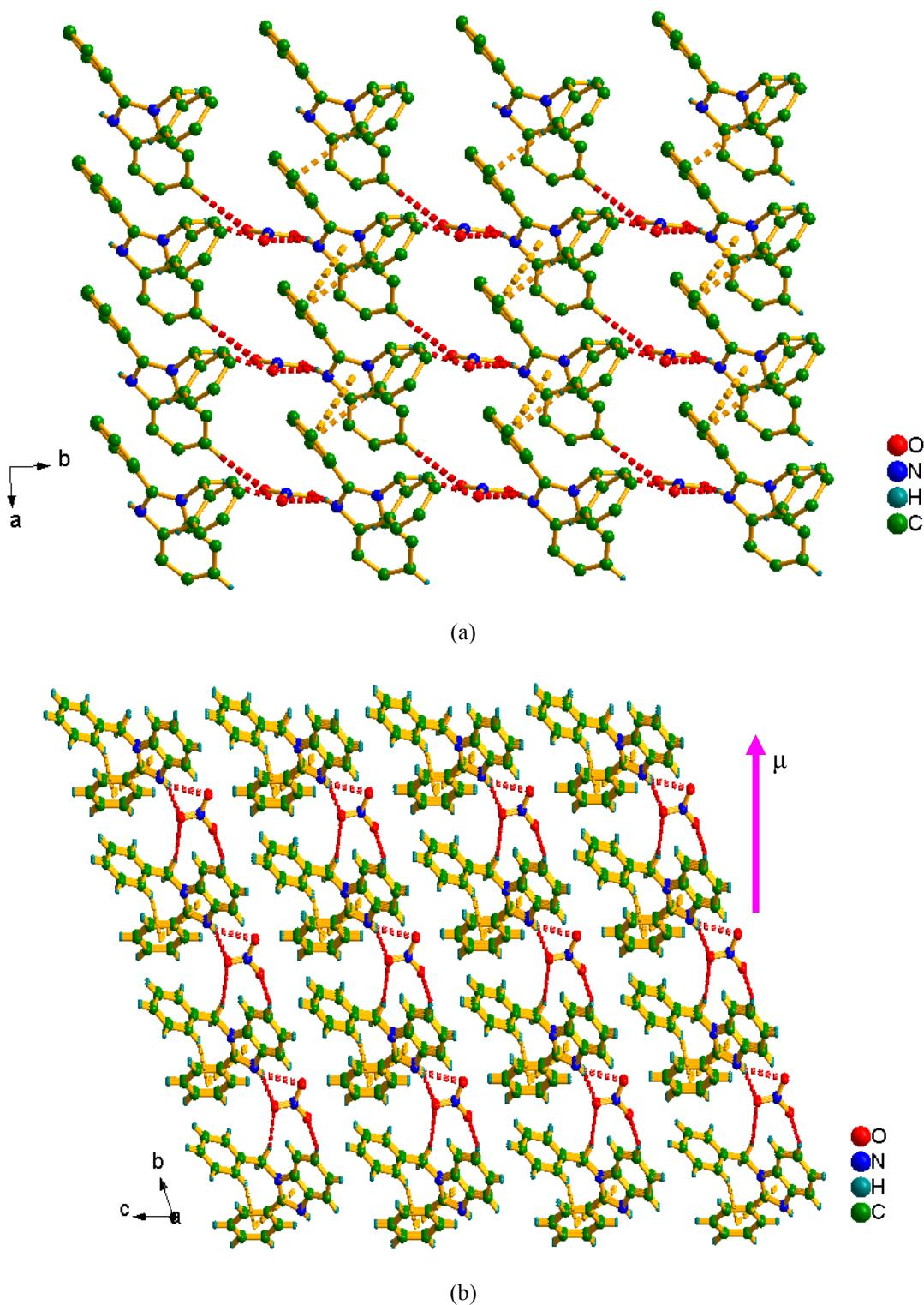
**Fig. S5** View point of 2D layer extending along the  $c$  axis in **2**. (b) Packing diagram of **2** along the  $a$  axis. The yellow dashed-lines and red ones represent  $\text{C}-\text{H}\cdots\pi$  and hydrogen bonds interactions, respectively. The thick yellow dashed-lines stand for  $\pi\cdots\pi$  packing interactions. The purple arrow stands for the direction of packing polar polarity.
