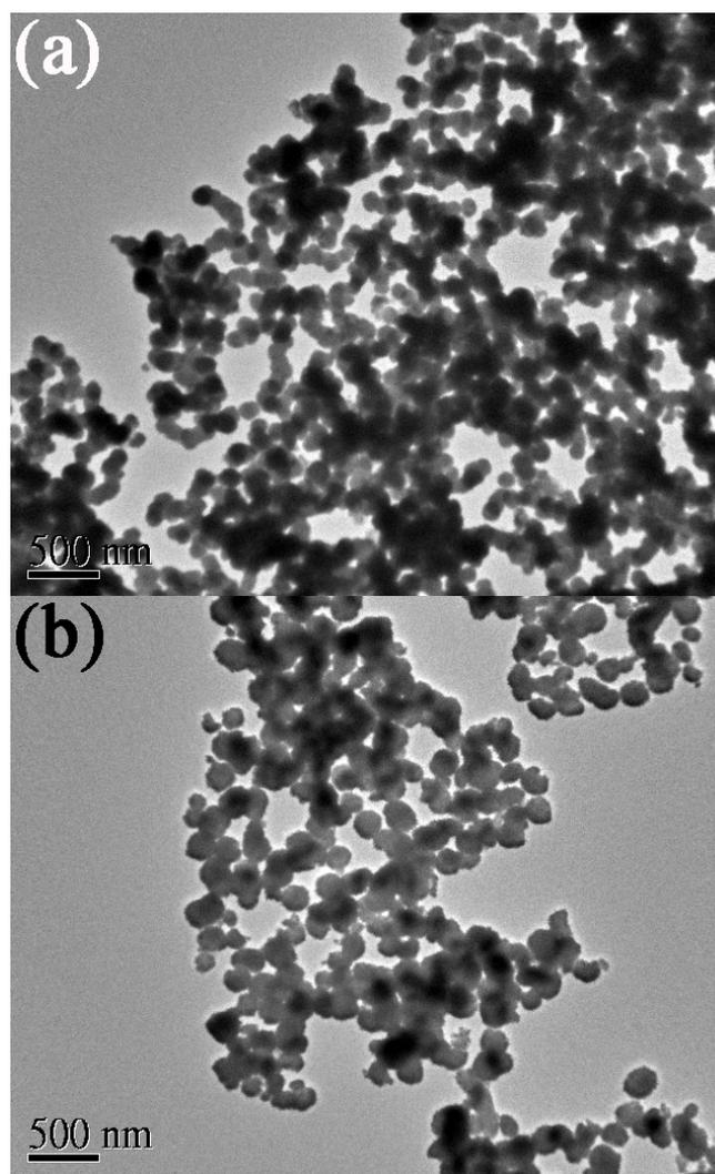
**Fig. S4** TEM images of bare Fe<sub>20</sub>Ni<sub>80</sub> prepared with different metal ion concentration:
