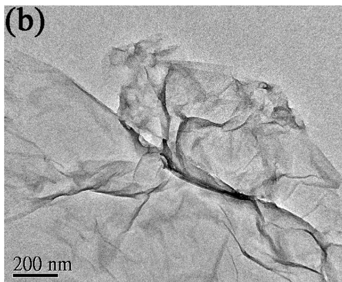
**Fig. S1** (a) XRD pattern and (b) TEM image of bare RGO nanosheets prepared in the absence of  $\text{FeSO}_4 \cdot 7\text{H}_2\text{O}$  and  $\text{NiCl}_2 \cdot 6\text{H}_2\text{O}$  with the same procedures.
