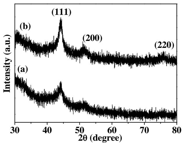
**Fig. S3** XRD patterns of RGO-Fe<sub>20</sub>Ni<sub>80</sub> composites with different metal ion concentration: (a) RGO-Fe<sub>20</sub>Ni<sub>80</sub>-1.4; (b) RGO-Fe<sub>20</sub>Ni<sub>80</sub>-5.6.
