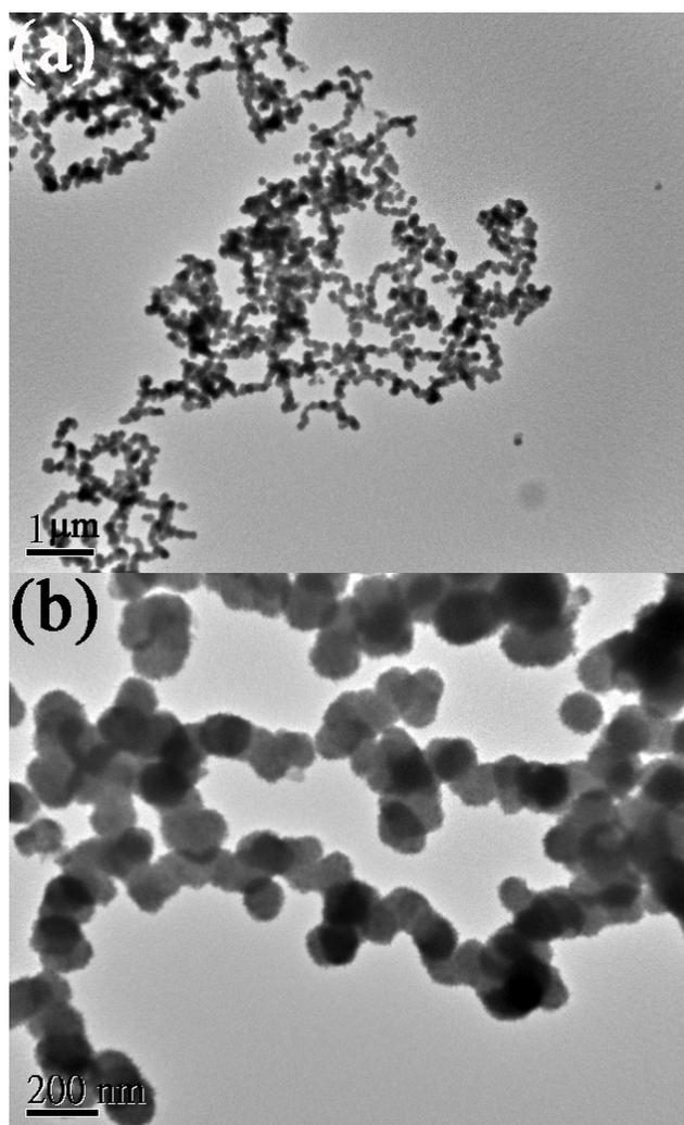
**Fig. S2** TEM images of the bare Fe<sub>20</sub>Ni<sub>80</sub> prepared with the same procedures of RGO-Fe<sub>20</sub>Ni<sub>80</sub>-2.8 nanoflowers ( $[\text{Fe}^{2+}] + [\text{Ni}^{2+}] = 2.8 \text{ mM}$ ) in the absence of GO.
