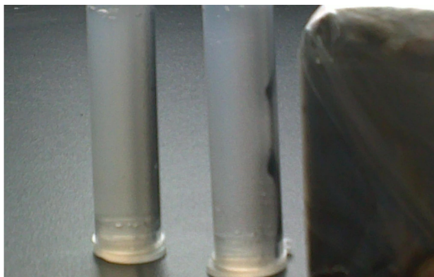
Figure S3. Visual image of FeCO 3 @Fe 3 O 4 nanoparticles (left) and flower-like assemblies (right) when an external magnet was applied.
