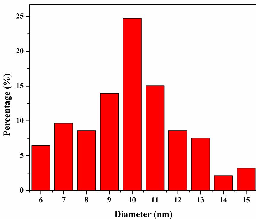
**Fig. S3** Histogram of nanoparticle size distribution of PbSnS nanocrystals ( $x=0.85$ ).
