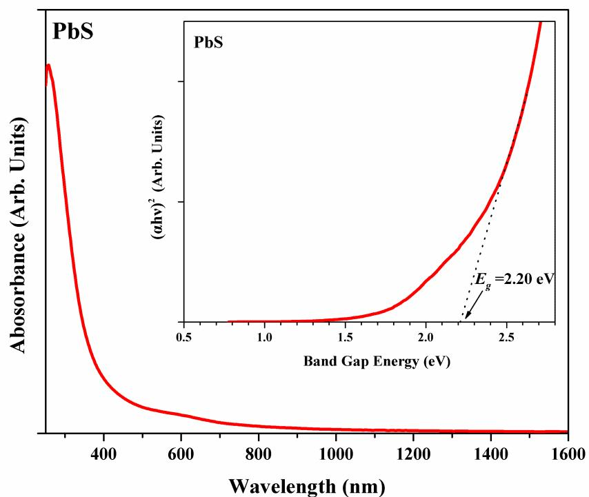
**Fig. S5** Abosorbance spectra of PbS nanocrystals and the obtained band gap energy (inset).
