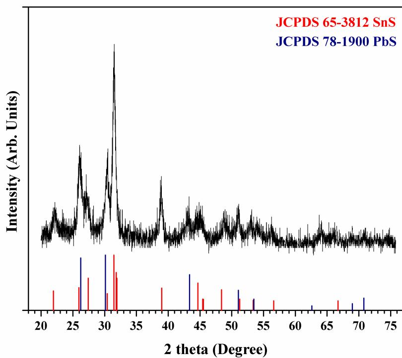
**Fig. S2** PbSnS nanocrystals sample with a secondary phase SnS (JCPDS 65-3812).
