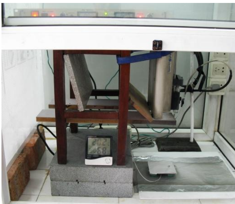
Figure S1. The setup of electrospinning used in our laboratory. The precision syringe pump (KDS-200, Stoelting, Wood Dale, IL) delivered the polymer precursor solution, and the voltage of electrospinning was maintained by a high-voltage power supply (Glassman High Voltage Inc. model Series FC with a positive polarity). As a high voltage was applied, the precursor solution jet accelerated towards the cathode with a 20-gauge blunt stainless steel needle tip, leading to the formation of the electrospun fiber nonwoven mats onto the Al foil placed over a grounded copper collector plate accompanied by partial solvent evaporation. Upon Co doping, the color of the buffer solution turns from colorless to pink.
