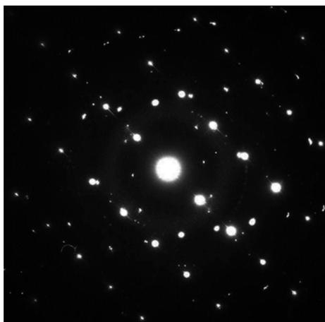
**Fig. S2** Selected area electron diffraction pattern from the SBN60-STO film-substrate interface. The indexed versions of this as-collected pattern are presented in Fig. 3.
