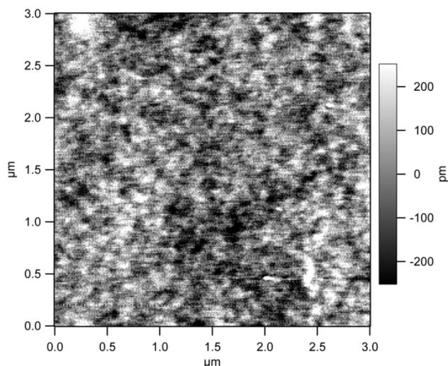
**Fig. S3** Atomic force microscopy surface scan of the SBN60 thin film surface over a  $3 \mu\text{m} \times 3 \mu\text{m}$  area.
