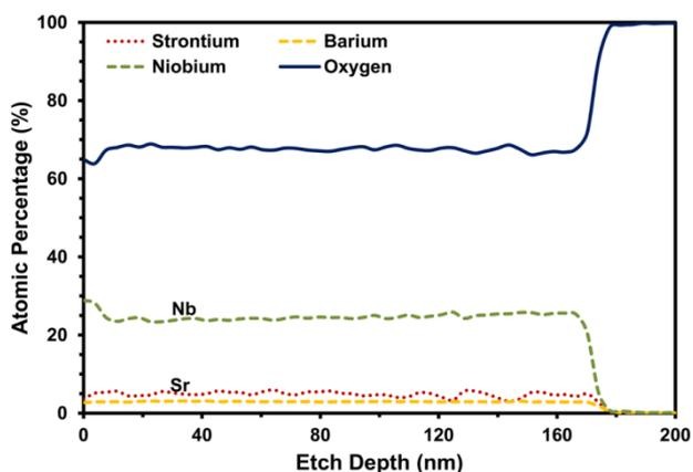
**Fig. S1** X-ray photoelectron spectroscopy depth profile of ~175 nm thick SBN60 film, as-deposited under conditions in Table S1.
