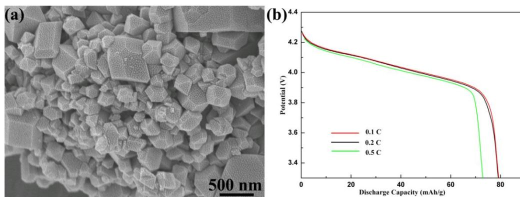
Fig. S5 (a) SEM of the  $LiMn_2O_4$  using  $Mn_3O_4$  nanocubes as raw material at  $750\text{ }^\circ\text{C}$  for 6h. (b) Discharge curves at 0.1 C, 0.2 C and 0.5 C, the capacity are 79.8, 79.2 and 72.9 mAh/g, respectively.
