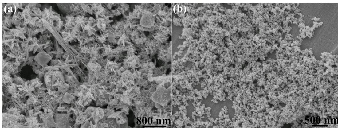
Fig. S4 The SEM images (a)  $N_2$  protecting, (b) excess  $O_2$ .
