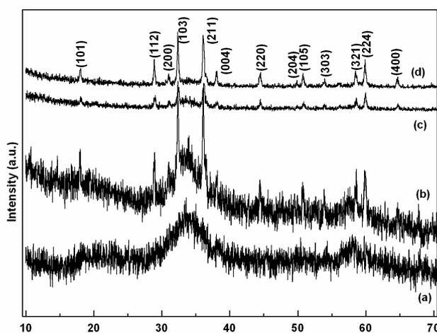
**Fig. S1** XRD patterns of products obtained at 200 °C for different reaction times: (a) 0.5 h, (b) 1.0 h, (c) 6 h and (d) 12 h.
