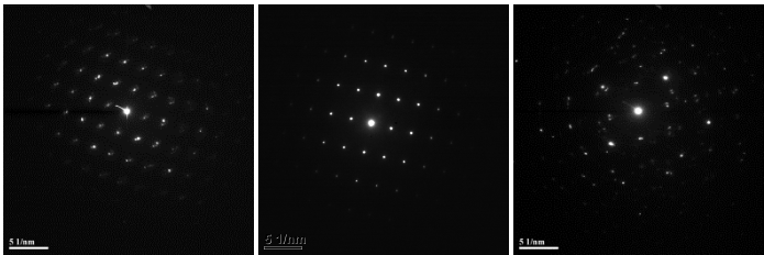
Figure S1. The corresponding electron diffraction patterns of cubic NiSe 2 , orthorhombic NiSe 2 and hexagonal NiSe.
