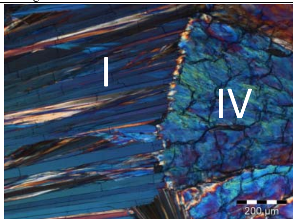
Fig. S3 Melt-film preparation showing NbtI-I (left) and NbtI-IV (right) produced by annealing the supercooled melt at about 70 °C
