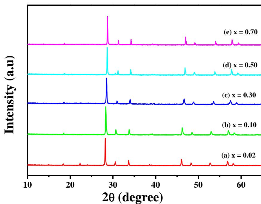
**Fig. S1** XRD patterns of  $\text{NaLa}_{1-x}(\text{MoO}_4)_2:x \text{ Eu}^{3+}$  samples prepared by hydrothermal method at  $180^\circ\text{C}$  for 12 h with different doping concentrations ( $x = 0.02, 0.10, 0.30, 0.50, 0.70$ ).
