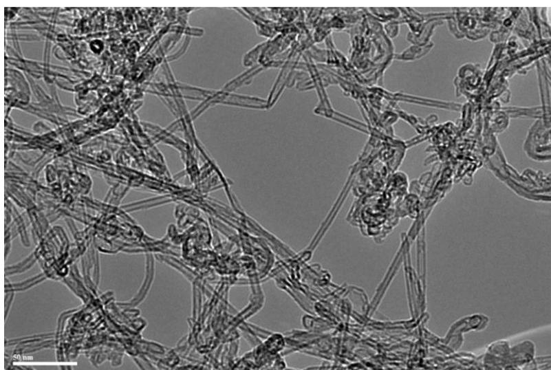
Figure S2: The TEM image of P-MWCNTs
