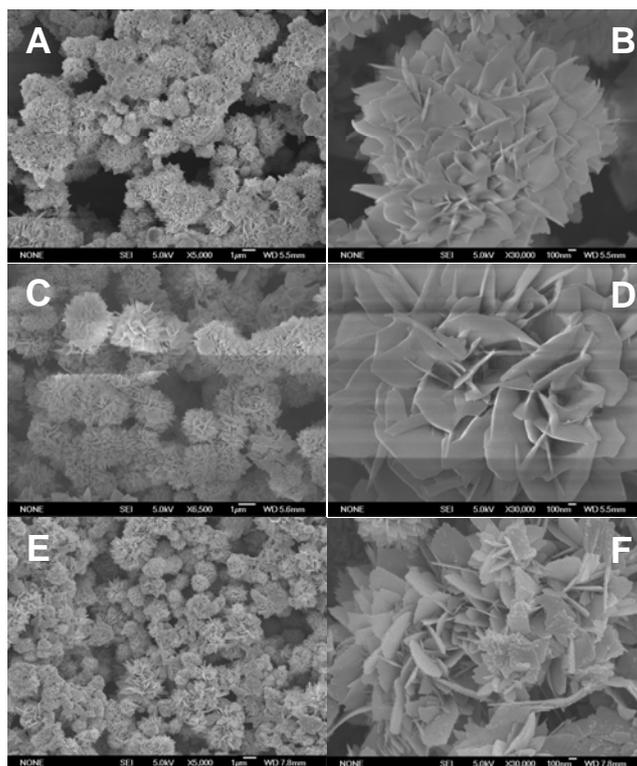
**Figure S3.** FESEM images of SnO<sub>2</sub> nanosheets prepared with different reaction durations while other conditions remained unchanged: (A, B) 5 h, (C, D) 10 h, (E, F) 30 h.
