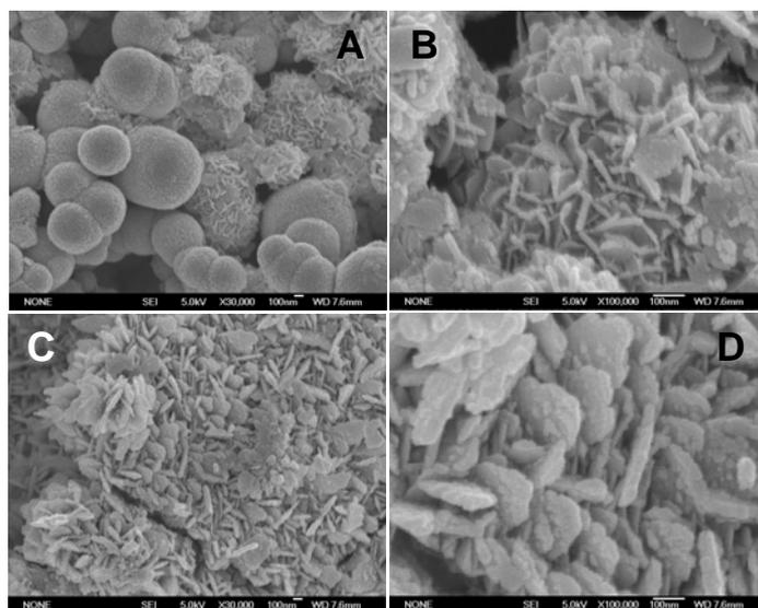
**Figure S2.** FESEM images of SnO<sub>2</sub> nanosheets prepared with different amounts of NH<sub>4</sub>F while other conditions remained unchanged: (A, B) 0.15 g, (C, D) 0.3 g.
