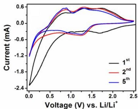
**Figure S5.** CV curves of SnO<sub>2</sub> NSs prepared without PVP.
