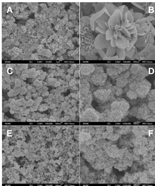
**Figure S4.** FESEM images of SnO<sub>2</sub> nanosheets prepared with different tin precursors while the concentrations of Sn and F ions, as well as other conditions remained unchanged: (A, B) SnF<sub>2</sub>, (C, D) SnCl<sub>4</sub>, (E, F) K<sub>2</sub>SnO<sub>3</sub>·3H<sub>2</sub>O.
