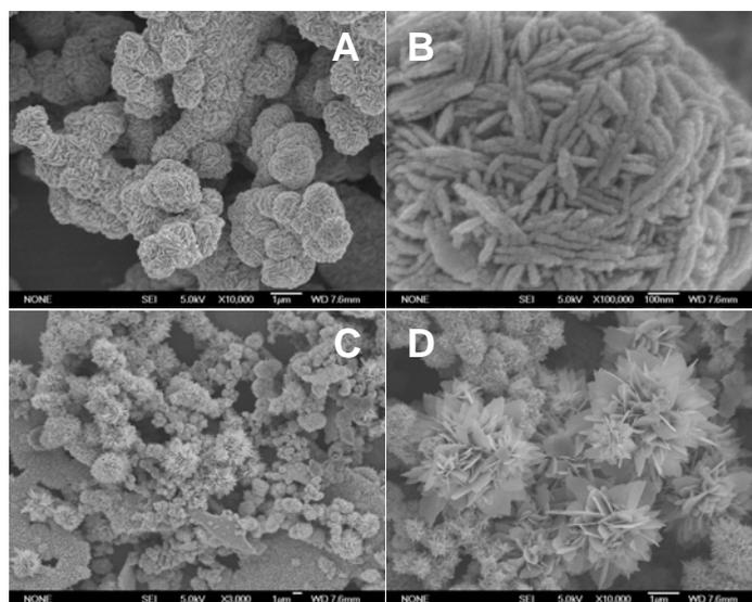
**Figure S1.** FESEM images of SnO<sub>2</sub> NSs prepared with different amounts of SnCl<sub>2</sub>·2H<sub>2</sub>O while other conditions remained unchanged: (A, B) 0.30 g, (C, D) 0.5 g.
