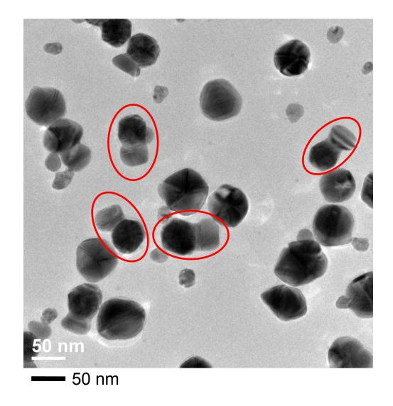
**Fig. S1**. TEM image of decahedral Au@Ag nanocrystals prepared under MW heating at an [Ag ]/[Au] atomic ratio of 7. Twin particles formed from icosahedral Au cores are shown by red circles.
