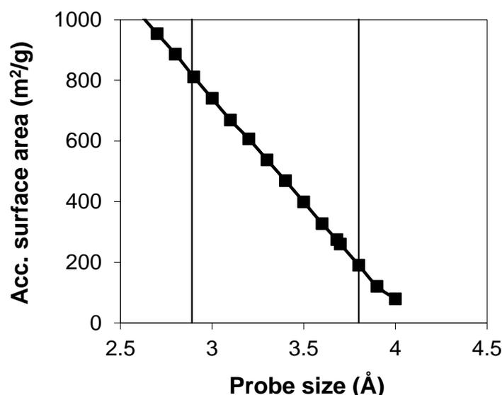
**Figure S3.** Accessible surface area of **2** obtained with different probe molecules with a diameter ranging between 2.6 and 4.0 Å. Vertical lines show the kinetic diameter of H<sub>2</sub> (2.89 Å) and CH<sub>4</sub> (3.8 Å), and so the accessible surface areas for this compound.
