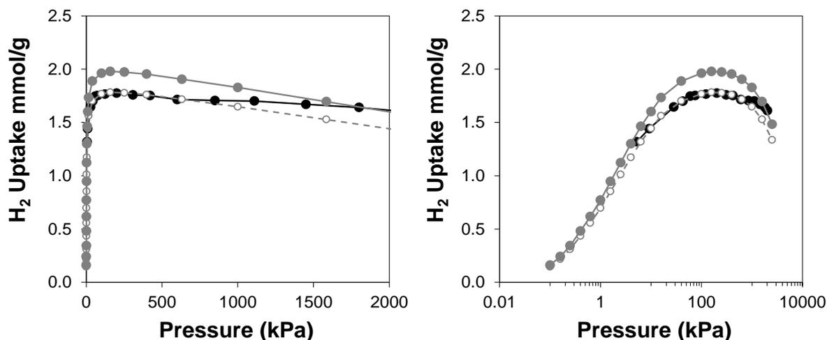
**Figure S4.** (*left*) Experimental, black closed circles, and simulated, grey closed circles, H<sub>2</sub> isotherms at 77 K on **2**. Scaled ( $\Pi = 0.91$ ) simulated isotherms, grey open circles. (*right*) Semilog representation of the H<sub>2</sub> isotherms.
