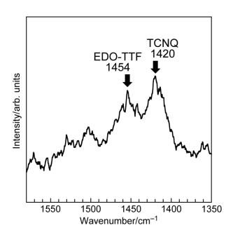
**Figure S2.** Raman spectrum of **1** with an excitation of 632.8 nm.
