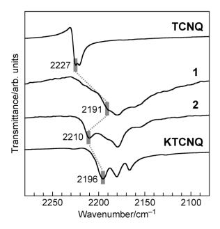
Figure S1.  $C\alpha N$  stretching modes in the IR spectra of 1, 2, TCNQ and KTCNQ salt measured in KBr pellets.
