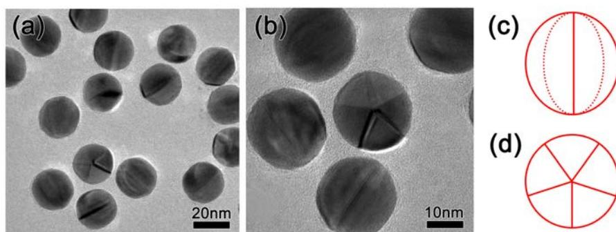
**Fig. S2** (a) and (b) TEM images of Seed 2. Because the twinned boundaries can't be focused at the same level along the non-axial direction, most of Seed 2 look like single-twined or single-crystalline structure. Illustrations of the twinned boundaries observed in the equatorial and axial direction are given in (c) and (d).
