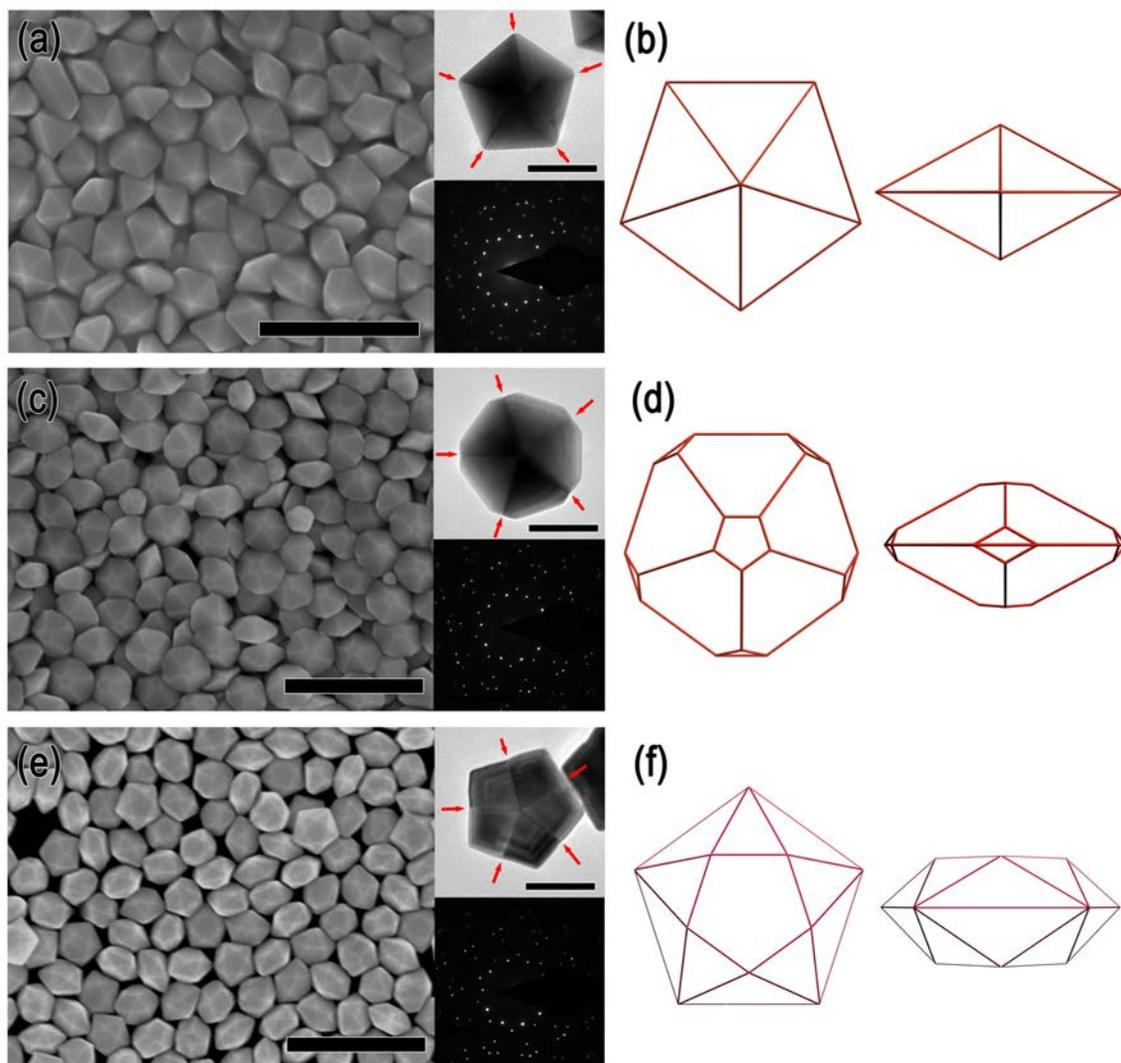
**Fig. S3** Typical SEM images (scale bars: 500nm), TEM images (top insets, scale bars: 100nm) and electron diffraction patterns (bottom insets) of the five-fold twinned (a) Dh, (c)TD, and (e) PS Au NCs. The red arrows indicate the twin boundaries. The wireframe of the five-fold twinned (b) Dh, (d) TD and (f) PS in the top view and side view. Twined boundaries aren't delineated in (d) and (f).
