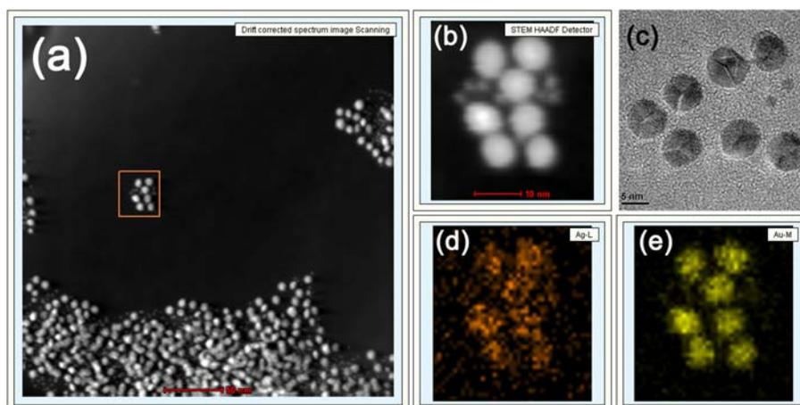
**Fig. S1** STEM images of Seed 1 in the scale bar of (a) 50nm and (b) 10nm. (c) A typical TEM image of Seed 1, in which five-fold twinned nanoparticles can be observed. (d) Ag and (e) Au element mapping images of Seed 1. The element mapping images demonstrate that Seed 1 are Au-Ag alloy rather than monometallic.
