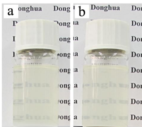
Fig. S4 Appearance of \text{TiO}_2 -OFG dispersed in water: (a) as-prepared and (b) one week later.
