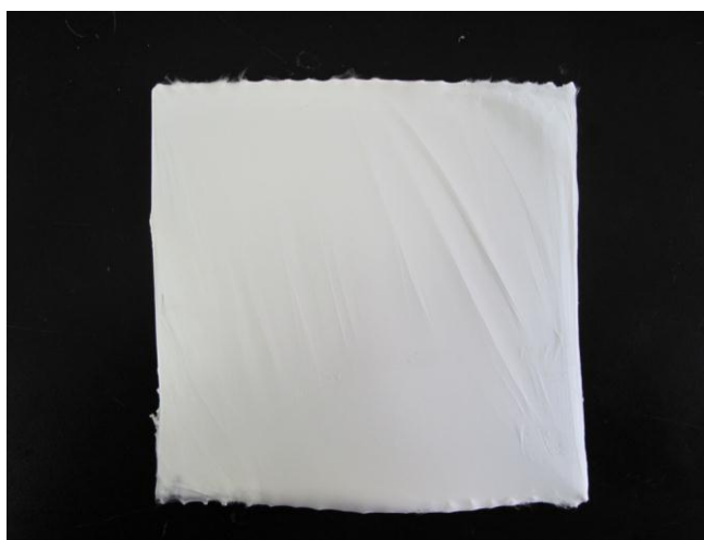
Fig. S1 Optical photo of the as-electrospun TiO 2 /PVP nanofibers similar with the one in the absence of TiO 2 .
