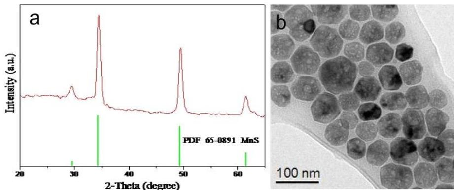
**Fig. S1** (a) XRD pattern, and (b) TEM micrograph of the synthesized cubic phase MnS nanocrystals.
