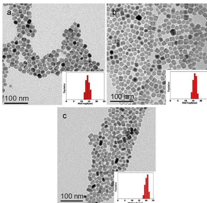
**Fig. S2**  $\text{Cu}_{1.94}\text{S}$ -MnS nanoheterostructures having reacted for (a) 10 min, (b) 15 min, and (c) 20 min respectively; insets of (a), (b) and (c) are the corresponding histograms by measuring 100 nanoheterostructures lying horizontally, showing MnS length distributions.
