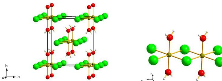
Fig. S9 Crystal structure of FeCl<sub>2</sub>·2H<sub>2</sub>O viewed along the c axis (left); detailed view of one edge-sharing chain (right)
