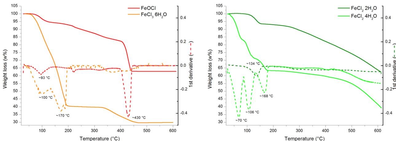
**Fig. S16** TGA diagrams (and their 1<sup>st</sup> derivative) of FeCl<sub>3</sub>·6H<sub>2</sub>O (orange line), FeOCl (red line) obtained by thermal treatment of FeCl<sub>3</sub>·6H<sub>2</sub>O, FeCl<sub>2</sub>·4H<sub>2</sub>O (green line) and FeCl<sub>2</sub>·2H<sub>2</sub>O (dark green line) obtained by thermal treatment of FeCl<sub>2</sub>·4H<sub>2</sub>O
