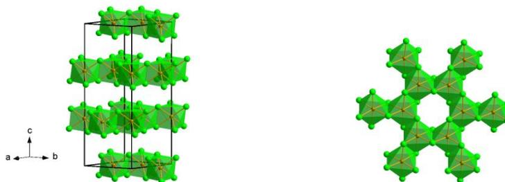
**Fig. S13** Crystal structure of FeCl<sub>3</sub> viewed along the [110] direction (left); detailed view of one layer showing the edge-sharing geometry (right)
