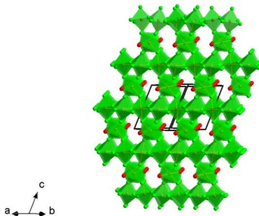
Fig. S6 Crystal structure of Fe<sub>3</sub>F<sub>8</sub>·2H<sub>2</sub>O viewed along the [110] direction
