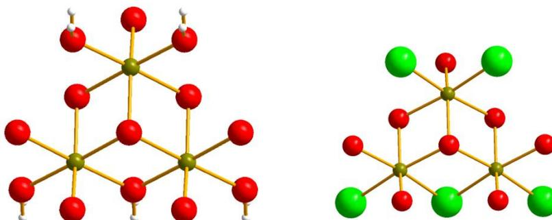
**Fig. S15** Comparison of the crystal structure of  $\gamma$ -FeOOH (left) and FeOCl (right); this shows the similarity between the two structures where the chlorides  $\text{Cl}^-$  and hydroxides  $\text{OH}^-$  occupy the same positions
