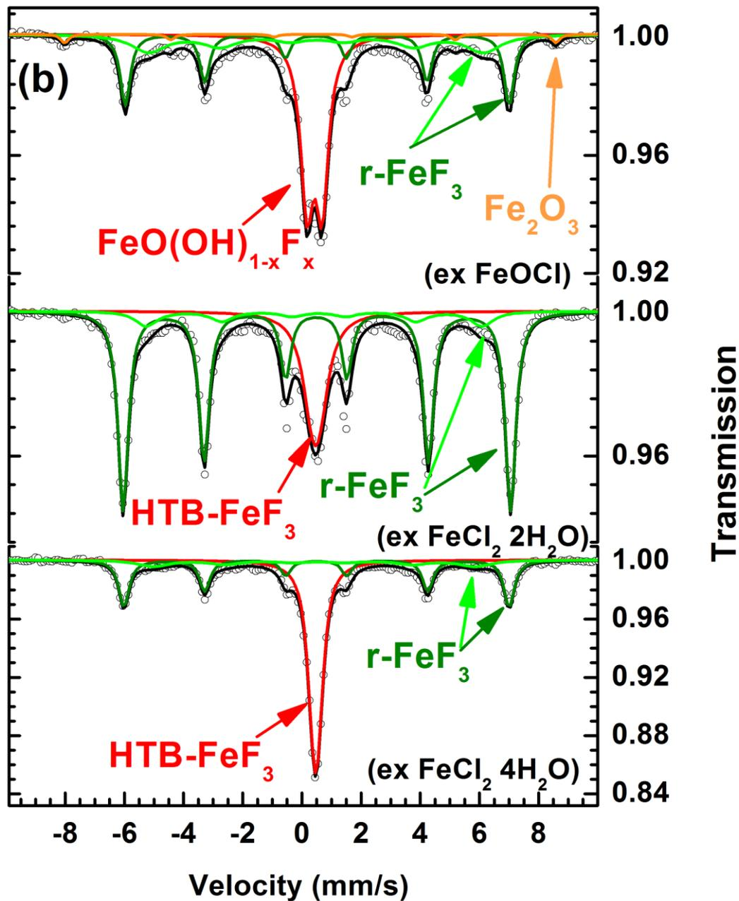
Fig. S20 Mössbauer spectra of the iron chloride precursors
