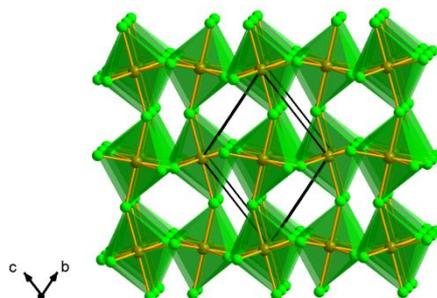
Fig. S1 Crystal structure of rhombohedral FeF<sub>3</sub> (r-FeF<sub>3</sub>) viewed along the *a* axis
