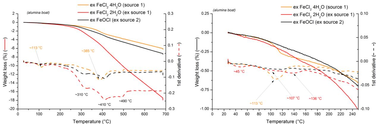
**Fig. S17** TGA diagrams of the fluorinated powders of FeCl<sub>2</sub>·4H<sub>2</sub>O (orange line), FeCl<sub>2</sub>·2H<sub>2</sub>O (red line) and FeOCl (black line), obtained by the one-shot procedure at 350 °C for 15 hrs (left); zoom on the range 25-250 °C (right)
