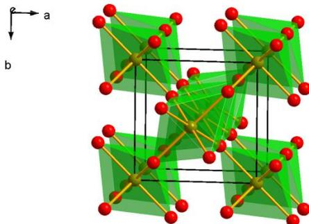
Fig. S7 Crystal structure of FeOF viewed along the *c* axis
