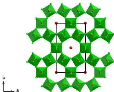
Fig. S2 Crystal structure of HTB FeF<sub>3</sub>·0.33H<sub>2</sub>O viewed along the *c* axis; the open channels where water molecules are accommodated are directed along the *c* axis
