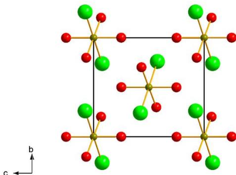
Fig. S8 Crystal structure of FeCl<sub>2</sub>·4H<sub>2</sub>O viewed along the *a* axis
