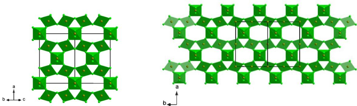
Fig. S3 Crystal structure of pyrochlore FeF<sub>3</sub> viewed along the [011] (left) and [0-11] directions (right), thus showing the 3D channels network
