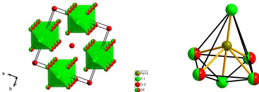
Fig. S4 Crystal structure of FeF<sub>3</sub>·3H<sub>2</sub>O viewed along the c axis (left); detailed geometry of the distorted Fe<sup>3+</sup> octahedra, showing the positional disorder of the oxygen and fluorine atoms around the iron (right)
