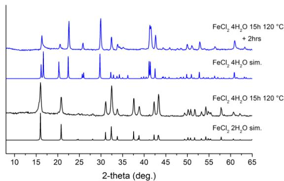
**Fig. S19** XRD patterns of  $\text{FeCl}_2 \cdot 4\text{H}_2\text{O}$  thermally treated under vacuum at 120 °C for 15 hrs, and the simulation of  $\text{FeCl}_2 \cdot 2\text{H}_2\text{O}$  (black line); the same powder exposed to air humidity for 2 hrs, and the simulation of  $\text{FeCl}_2 \cdot 4\text{H}_2\text{O}$  (blue line)
