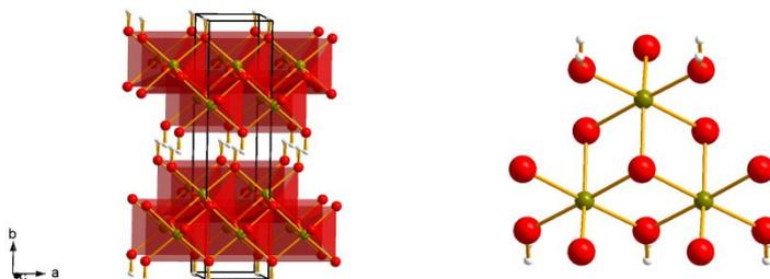
**Fig. S14** Crystal structure of  $\gamma$ -FeOOH viewed along the  $c$  axis (left); detailed view of one layer showing the edge-sharing geometry (right)
