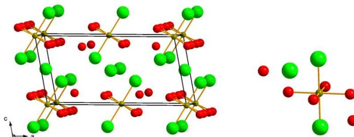
**Fig. S11** Crystal structure of FeCl<sub>3</sub>·6H<sub>2</sub>O viewed along the *b* axis (left); asymmetric unit (right)
