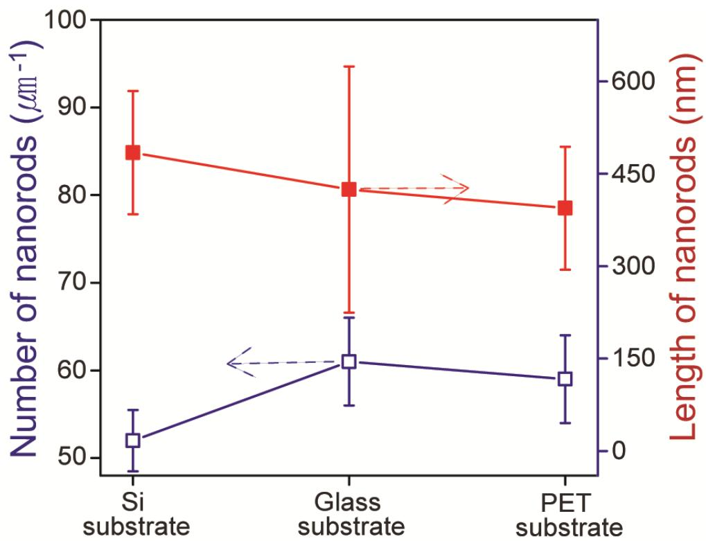
Figure S3. The population (the left-hand vertical axis) and length (the right-hand vertical axis) of ZnO nanorods grown for 5 h on different substrates.
