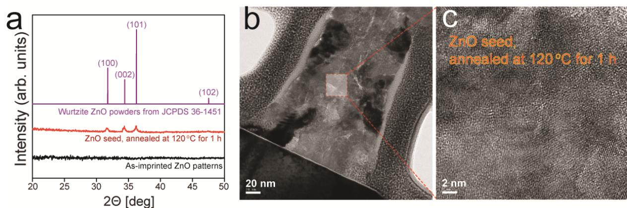
Figure S1. (a) XRD spectra of the as-imprinted ZnO patterns, the ZnO seed (i.e., the ZnO patterns etched with Cl<sub>2</sub> plasma followed by annealing at 120 °C for 1 h), and the standard power diffraction pattern of a wurtzite ZnO powder from JCPDS 36-14561. (b) A cross-sectional TEM image of the ZnO seed. (c) A high resolution TEM image obtained from the region highlighted by the dotted box in (b).
