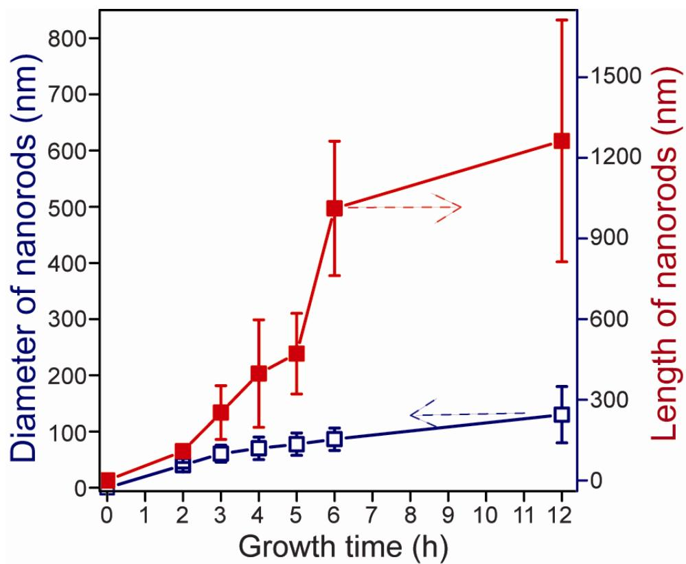
Figure S2. Dependences of ZnO nanorod diameter (the left-hand vertical axis) and length (the right-hand vertical axis) on the growth time.
