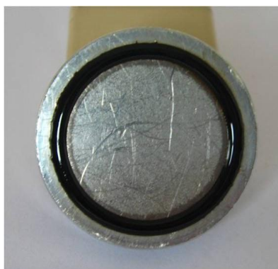
Figure S2. Photographs of loudspeaker use paraffin based magnetic fluid (cubic Fe 3 O 4 NCs) with 1 T
