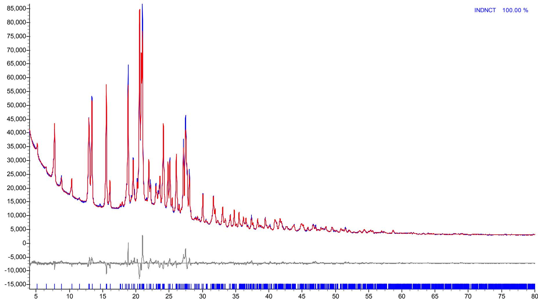
Profile plot of Rietveld fit to the IND:NIC diffraction data - 5-30°
