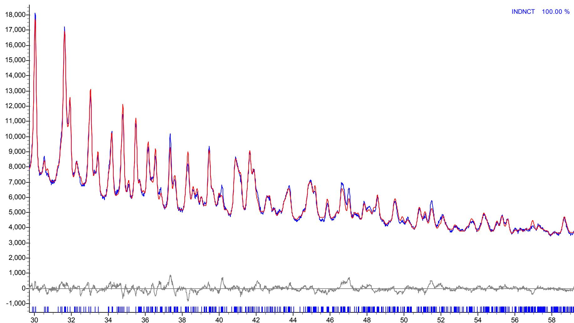
Profile plot of Rietveld fit to the IND:NIC diffraction data - 60-80° (difference plot omitted for clarity)
