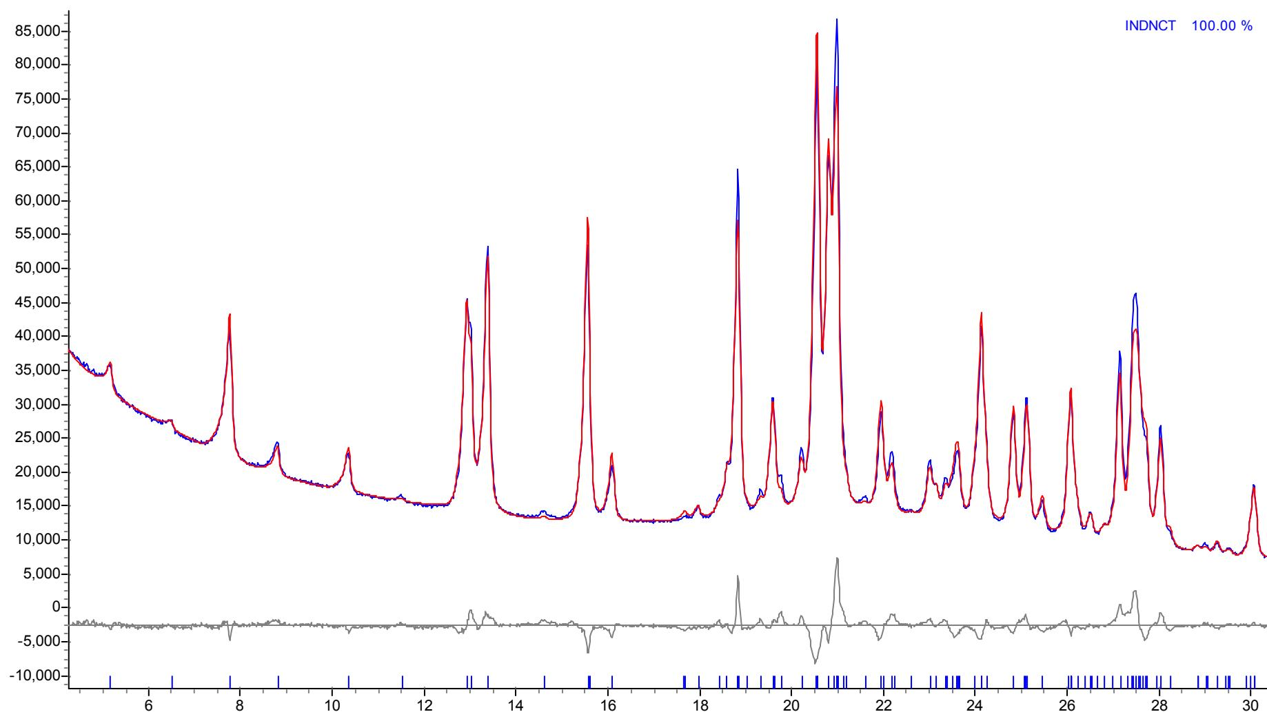
Profile plot of Rietveld fit to the IND:NIC diffraction data - 30-60°
