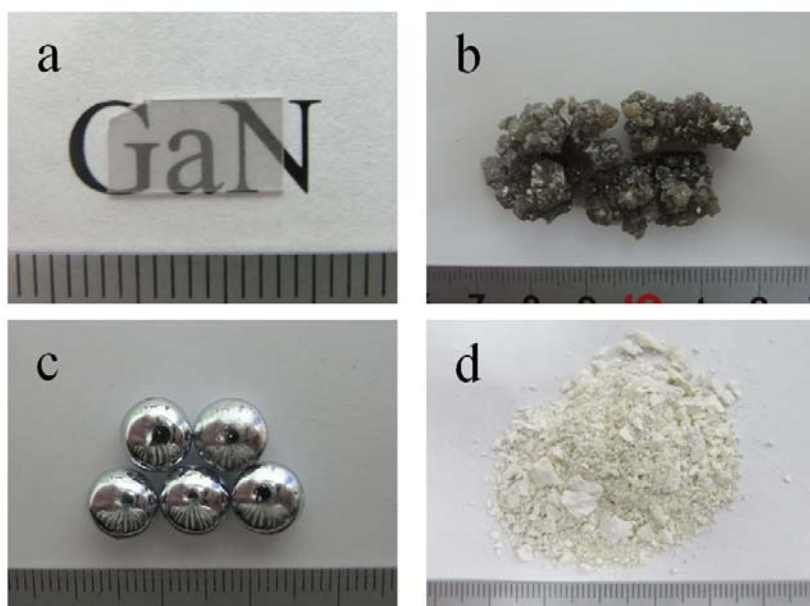
Figure 5. Images of HVPE seed and different nutrients. (a) HVPE seed; (b) polycrystalline GaN; (c) Ga metal; (d) GaN powder.
