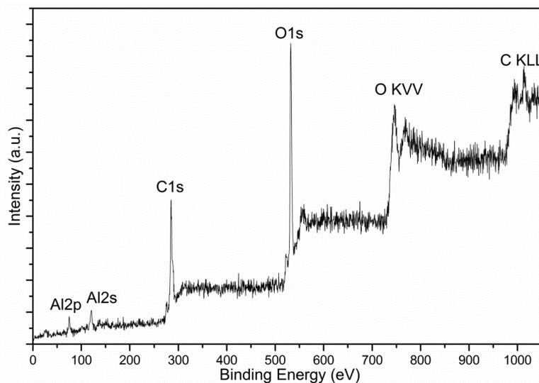
Figure S2. XPS spectrum of MIL-110 nanorod arrays as shown in Figure 1b.
