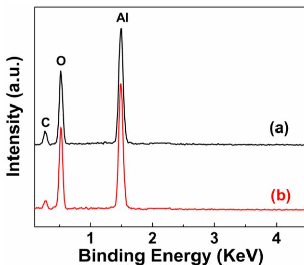
**Figure S5.** EDS of the samples prepared by putting thin films filtered from (a) 30ml cadmium hydroxide nanostrands , (b) 30ml zinc hydroxide in 30 ml, 1mM H<sub>3</sub>BTC aqueous solution at 120°C for 24h, respectively.
