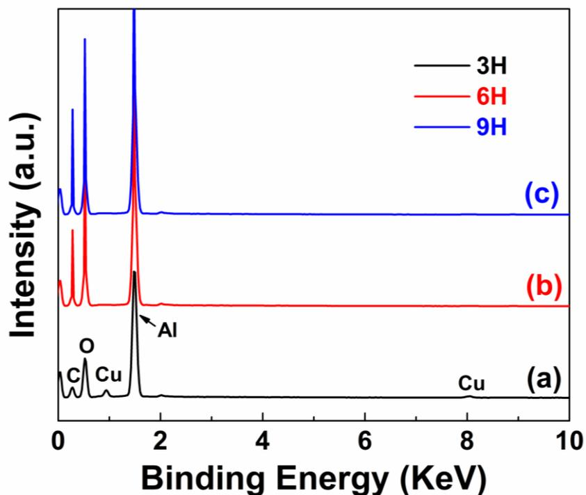
Figure S3. X-ray Energy dispersive analysis spectra of the samples prepared by putting CHNs thin films filtered from 30ml CHNs solution in 30 ml, 1mM H<sub>3</sub>BTC aqueous solution at 120°C for (a) 3 h, (b) 6 h, (c) 9 h, respectively.
