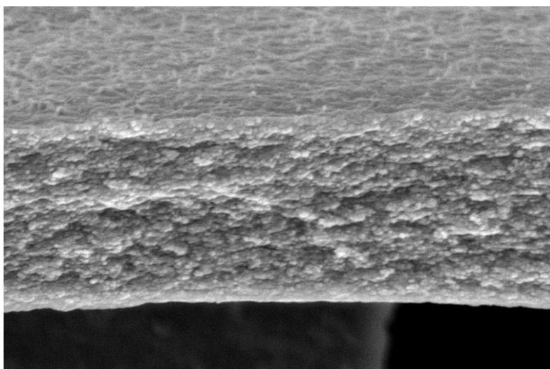
**Figure S1.** Cross-section SEM image of the CHNs thin films filtered from 30 ml CHNs solution on PC membrane with effective diameter of 1.9 cm.
