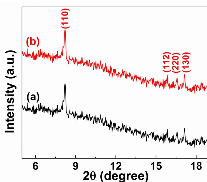
**Figure S6.** XRD of the samples prepared by putting thin films filtered from (a) 30ml cadmium hydroxide nanostrands , (b) 30ml zinc hydroxide in 30 ml, 1mM H<sub>3</sub>BTC aqueous solution at 120°C for 24h, respectively.
