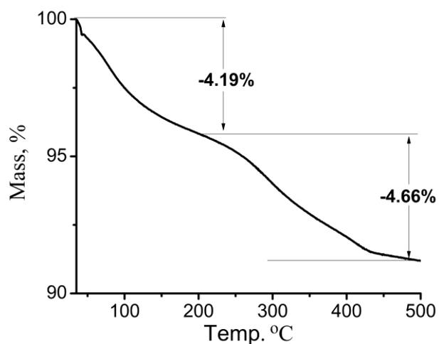
Figure S6 Weight change vs temperature for TG analysis of the microsphere performed at 10 °C/min up to 500 °C in flowing O<sub>2</sub>.
