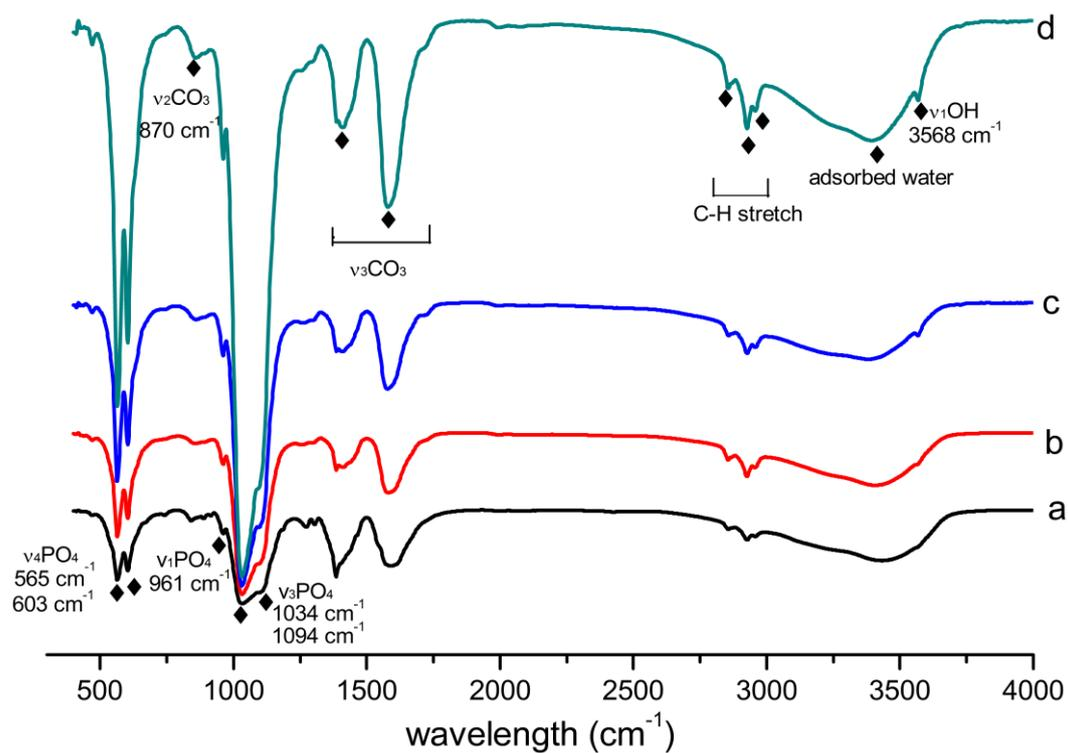
Figure S3 FT-IR patterns of products obtained after different reaction durations, a 25 min, b 30 min, c 40 min, d 60 min.
