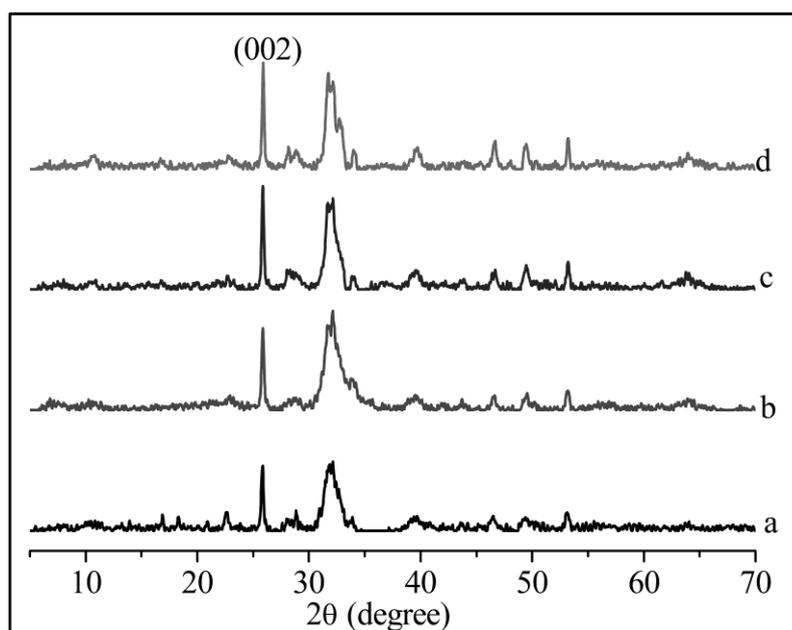
Figure S2 XRD patterns of products obtained after different reaction durations, a 25 min, b 30 min, c 40 min, d 60 min.
