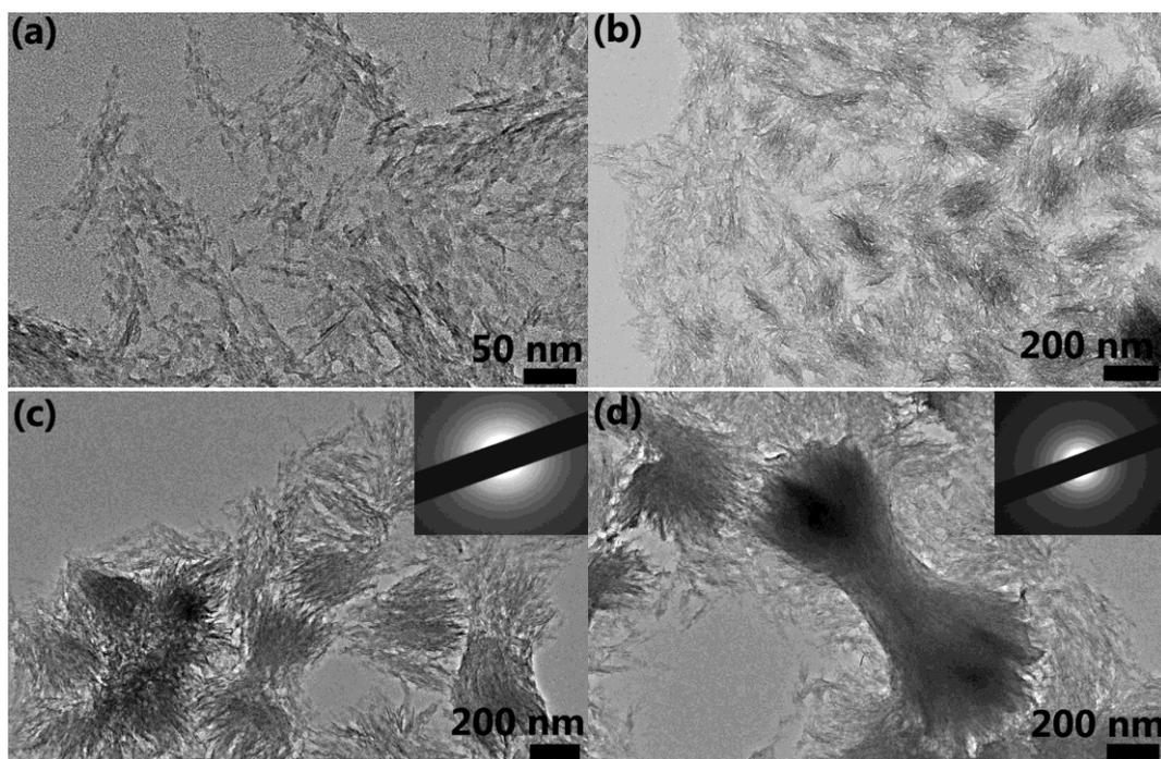
Figure S4 TEM images of progressive stages of the self-assembled growth of the precursor phase of HAp: from nanowires through paralleling mutually to dumbbell shapes calcium phosphate with low crystallinity.
