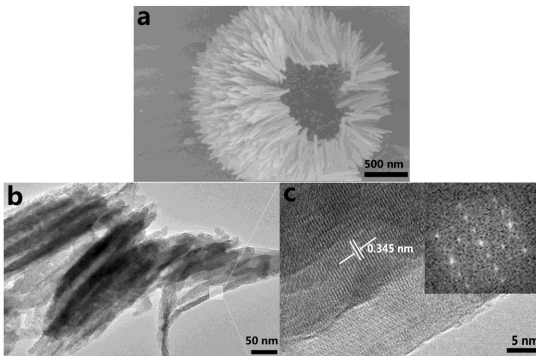
Figure S1 The SEM image of (a) MHAp and TEM image of (b) its building blocks, (c) the HRTEM images of the nano rod. The inset in (c) shows the corresponding FFT diffraction pattern.
