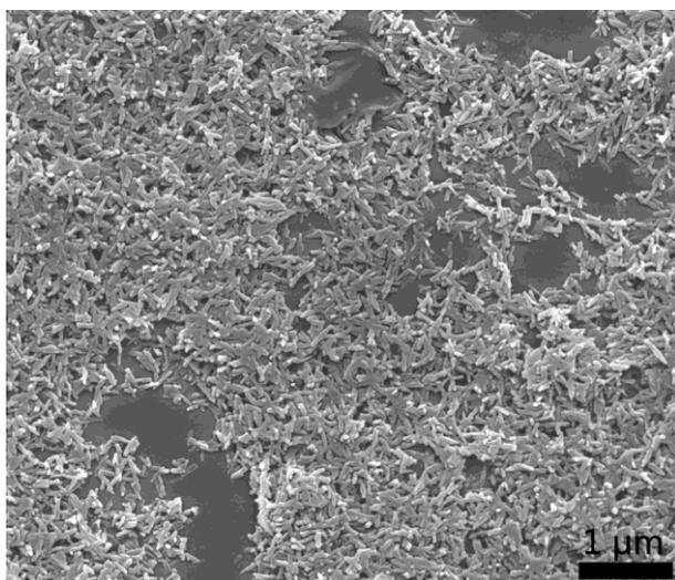
Figure S5 SEM image of HAp prepared at 180 °C for 2 h with the initial pH value at 6.4 and without adding sodium citrate. The synthesizing condition and the concentration of reagents was the same as the system of microsphere.
