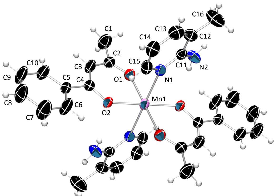
Figure S5. ORTEP plot of **V**. Thermal ellipsoids are shown with 50% probability and hydrogen atoms as spheres of arbitrary radius.
