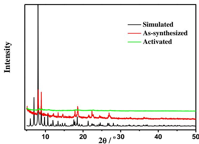
**Fig. S3.** X-ray powder diffraction patterns of MOF 2. Note that some differences in intensities between the calculated and experimental patterns may be due to the variation in crystal orientation or framework deterioration in the powdered samples.
