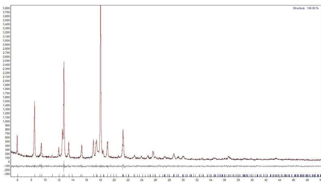
**Fig. S2.** Profile fitting of X-ray powder diffraction pattern of as-synthesized MOF 1. The red, blue, and gray lines are the calculated, the as-synthesized and the difference between the calculated and the as-synthesized. The blue bars are the calculated brag positions. The best fitting results for **1**:  $a = 29.467(6)$ ,  $c = 10.122(3)$ .
