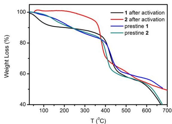
**Fig. S8.** TGA curves of MOFs **1** and **2**. Note that the activated **1** was left in air for several days before the TGA measurement.
