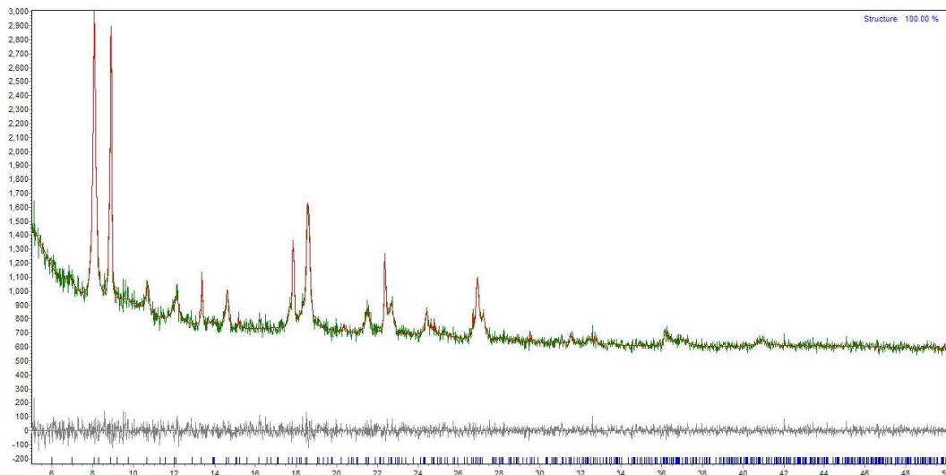
**Fig. S4.** Profile fitting of X-ray powder diffraction pattern of as-synthesized MOF 2. The red, black, and gray lines are the calculated, the as-synthesized and the difference between the calculated and the as-synthesized. The blue bars are the calculated brag positions. The best fitting results for 2:  $a = 25.321(51)$ ,  $c = 19.911(66)$ .
