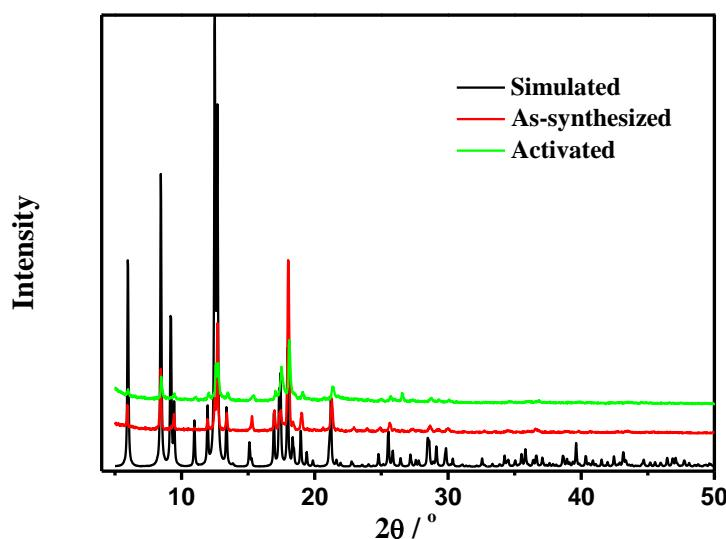
**Fig. S1.** X-ray powder diffraction patterns of MOF **1**. Note that some differences in intensities between the calculated and experimental patterns may be due to the variation in crystal orientation or framework deterioration in the powdered samples.
