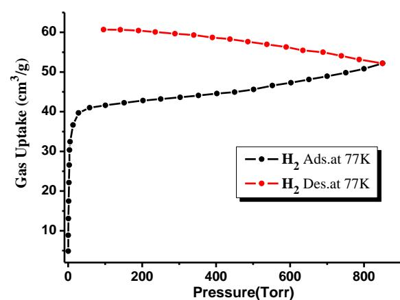
**Fig. S9** H<sub>2</sub> gas sorption isotherms of MOF 1 at 77 K.
