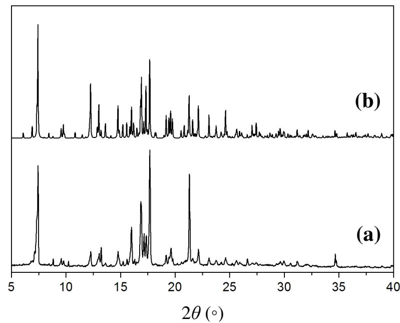
**Fig. S14** X-Ray powder diffraction (XRPD) patterns of **2**: (a) a freshly grounded sample at room temperature; (b) simulated from the single-crystal data. The sample of compound **2** was contained a small amount of compound **3**, making the experimental and simulated XRPD patterns do not fit quite well.
