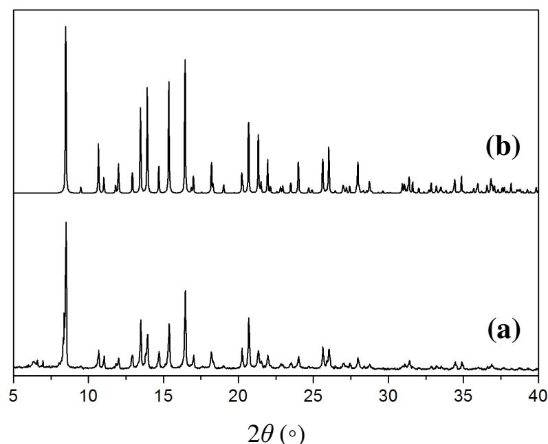
**Fig. S16** X-Ray powder diffraction (XRPD) patterns of **4**: (a) a freshly grounded sample at room temperature; (b) simulated from the single-crystal data.
