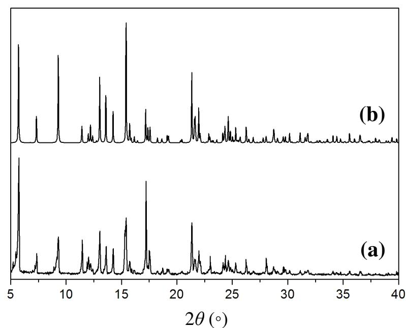
**Fig. S13** X-Ray powder diffraction (XRPD) patterns of **1**: (a) a freshly grounded sample at room temperature; (b) simulated from the single-crystal data.
