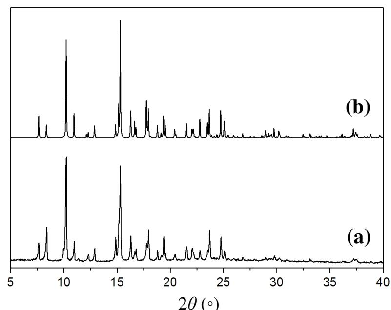
**Fig. S15** X-Ray powder diffraction (XRPD) patterns of **3**: (a) a freshly grounded sample at room temperature; (b) simulated from the single-crystal data.
