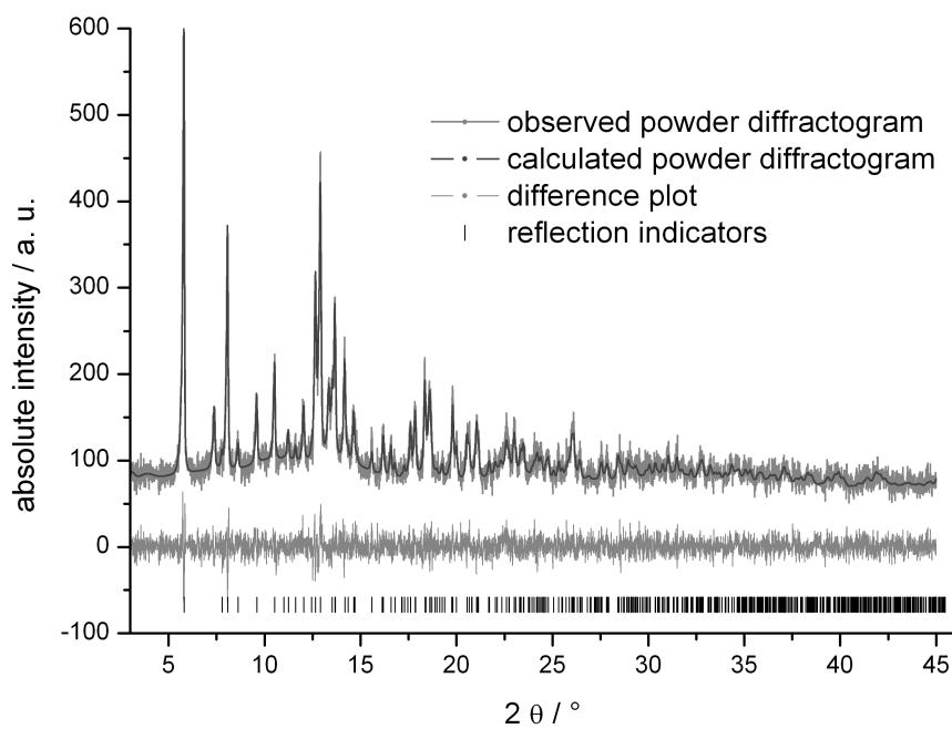
**Figure S1:** Observed (upper gray line) and calculated (black line) powder X-ray diffractograms from  $3^\circ$  to  $46^\circ$  ( $2\text{-theta}$ ) with difference plot from Rietveld refinement (lower gray line). Reflection positions are given as vertical black lines (bottom).
