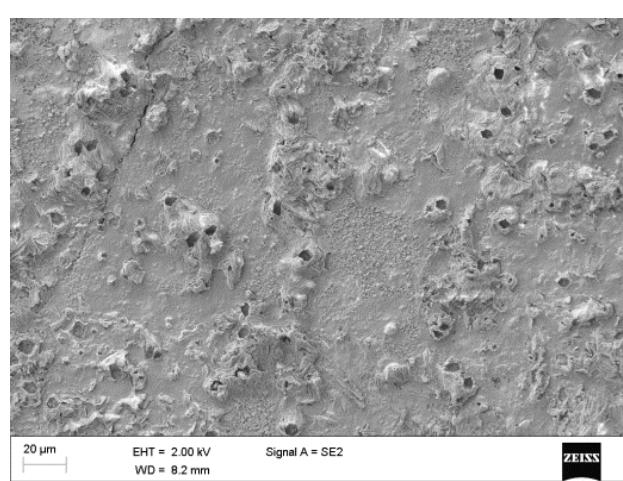
**Figure S3:** Scanning electron microscopy images of AAO (pore diameter 400 nm; pore depth 100  $\mu\text{m}$ ) coated with  ${}^3_{\infty}[\text{Sr}_{0.5}\text{Eu}_{0.5}(\text{Im})_2]$  from melt synthesis.
