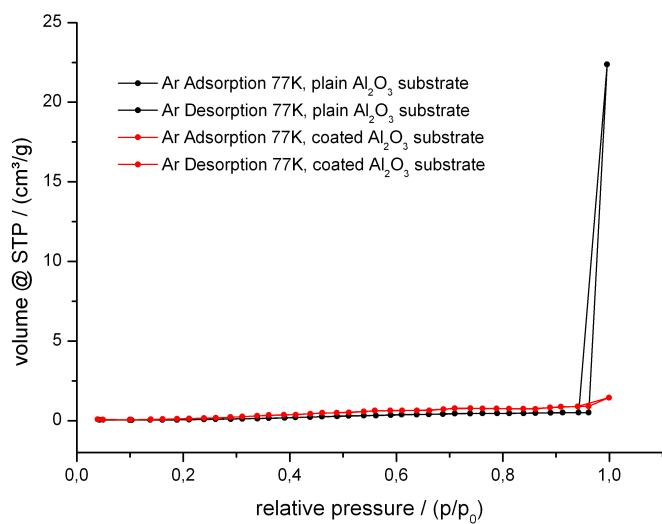
**Figure S7:** Argon adsorption on plain and coated AAO membranes (pore diameter 400 nm, pore depth 100 μm) according to the BET theory.
