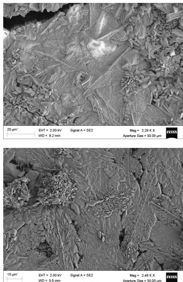
**Figure S5:** Scanning electron microscopy images of AAO (pore diameter 400 nm; pore depth 100  $\mu\text{m}$ ) coated with  $^3_{\infty}[\text{Eu}(\text{Im})_2]$  from melt synthesis.
