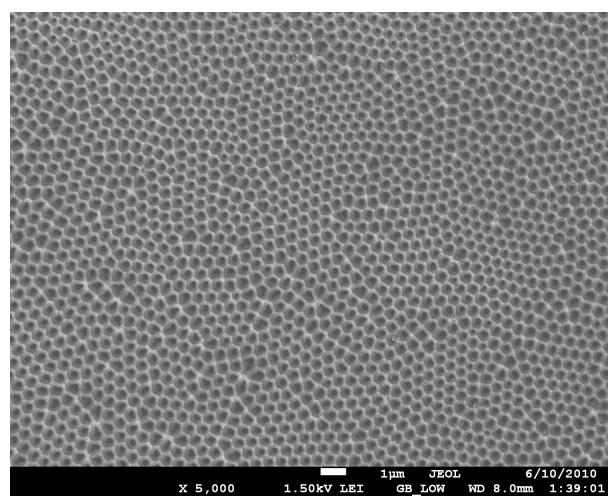
**Figure S2:** Top view scanning electron microscopy image of AAO having a pore diameter of 400 nm and a pore depth of 100 μm.
