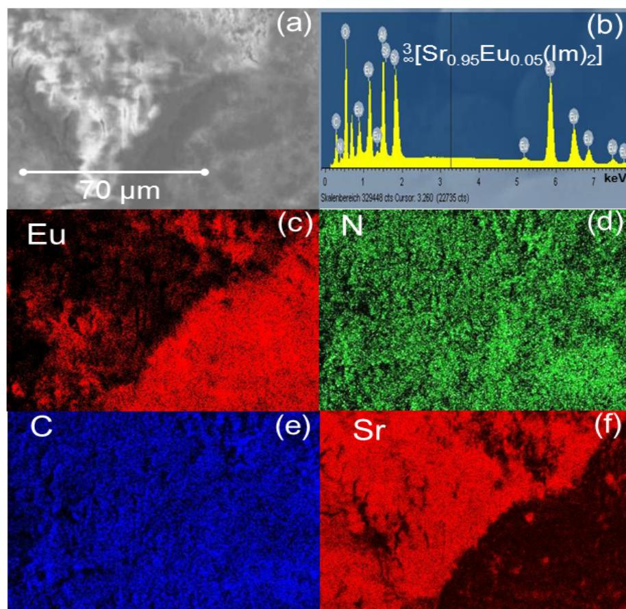
**Figure S6:** SEM and EDX element mapping of  ${}^3\infty[\text{Sr}_{0.95}\text{Eu}_{0.05}(\text{Im})_2]$  from liquid ammonia
