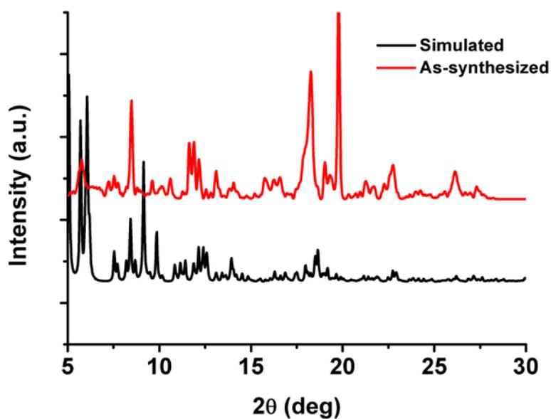
**Fig. S2** Powder X-ray diffraction patterns of MMPF-8.
