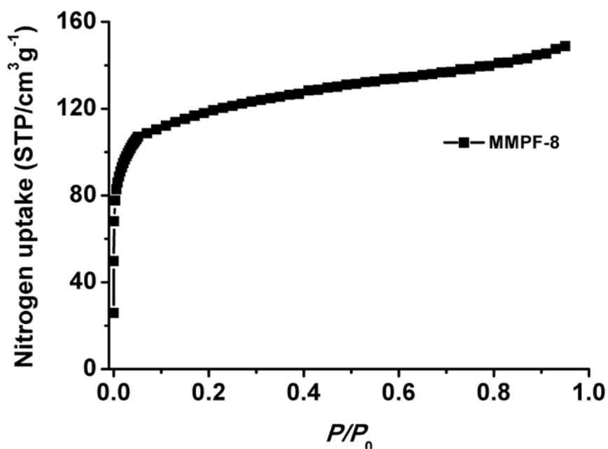
Fig. S4 Nitrogen isotherm of MMPF-8 at 77K.
