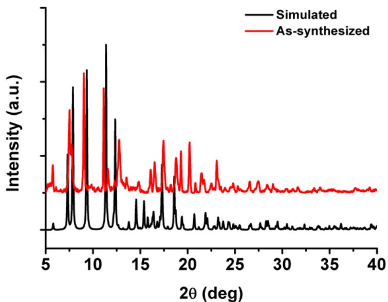
**Fig. S1** Powder X-ray diffraction patterns of MMPF-7.
