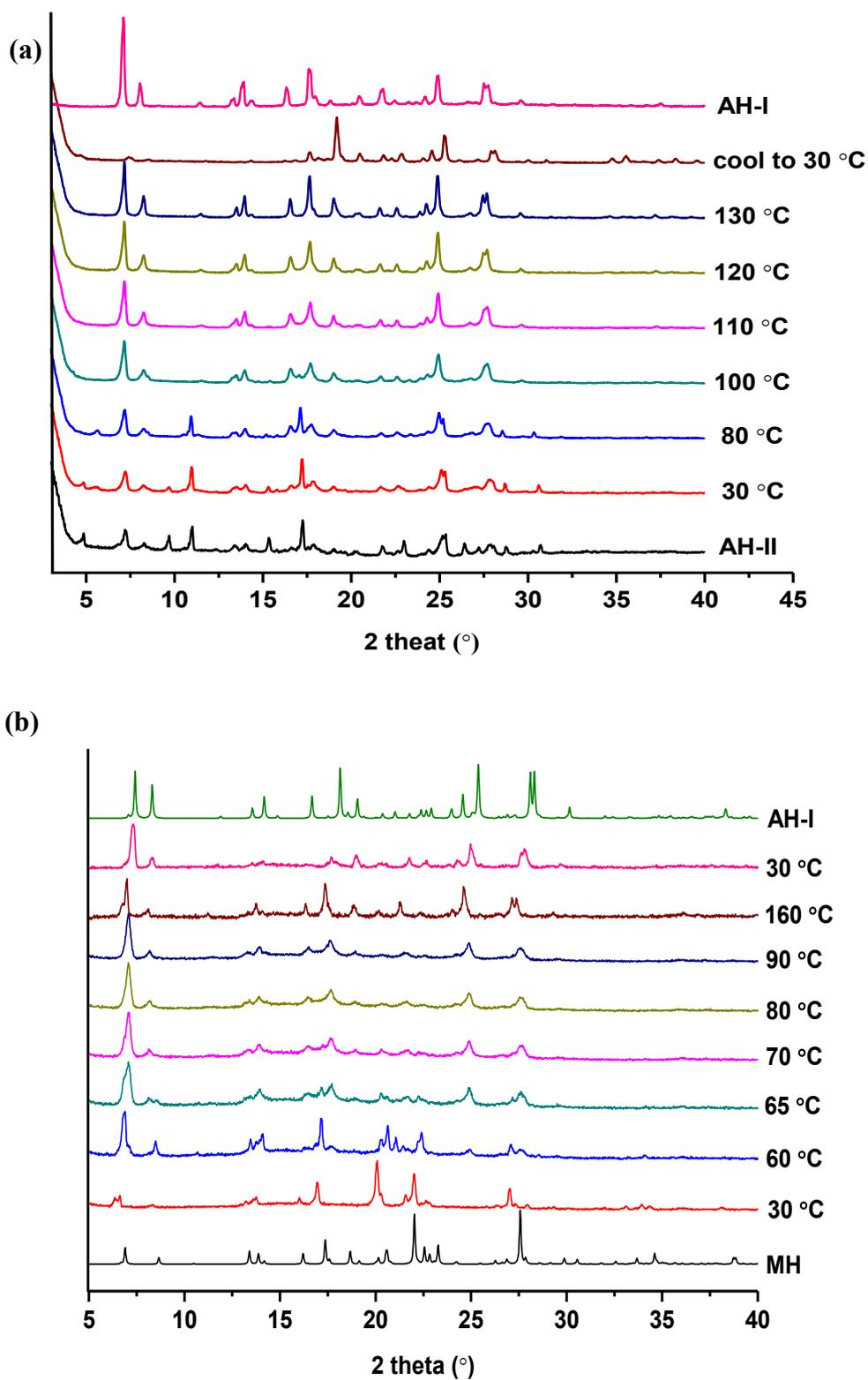
Fig. S5 VT-XRPD pattern of AH-II (a) and MH (b).
