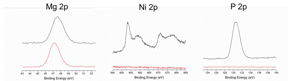
Figure S3.1 XPS spectra of unmodified (red) and with 10 % nickel and  $\text{H}_3\text{PO}_4$  modified CPO-27(Mg) (black).
