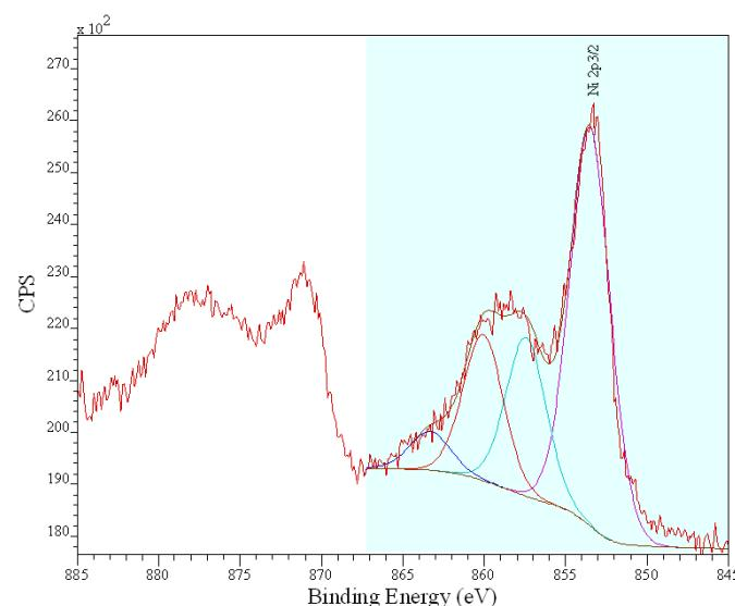
Figure S3.2 XPS spectra of 10 % nickel and  $\text{H}_3\text{PO}_4$  modified CPO-27(Mg) with applied fitting parameters in Ni 2p<sub>3/2</sub> region.<sup>11</sup>
