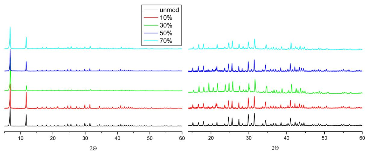
Figure S4.1 PXRD of unmodified CPO-27 (Mg) and with various amounts of *cpmp* and  $\text{Ni}^{2+}(\text{aq})$  modified material. Powder patterns were collected after activation at 373 K followed by 523 K and adsorption experiments.
