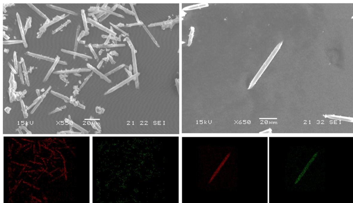
Figure S8.2 Elemental maps of CPO-27(Mg) modified with 70%  $\text{Ni}^{2+}$  and 10% *cpmp* recorded after different second step reaction times. 1 hour (left), 3 days(right). (Mg Ka, red; Ni Ka, green)
