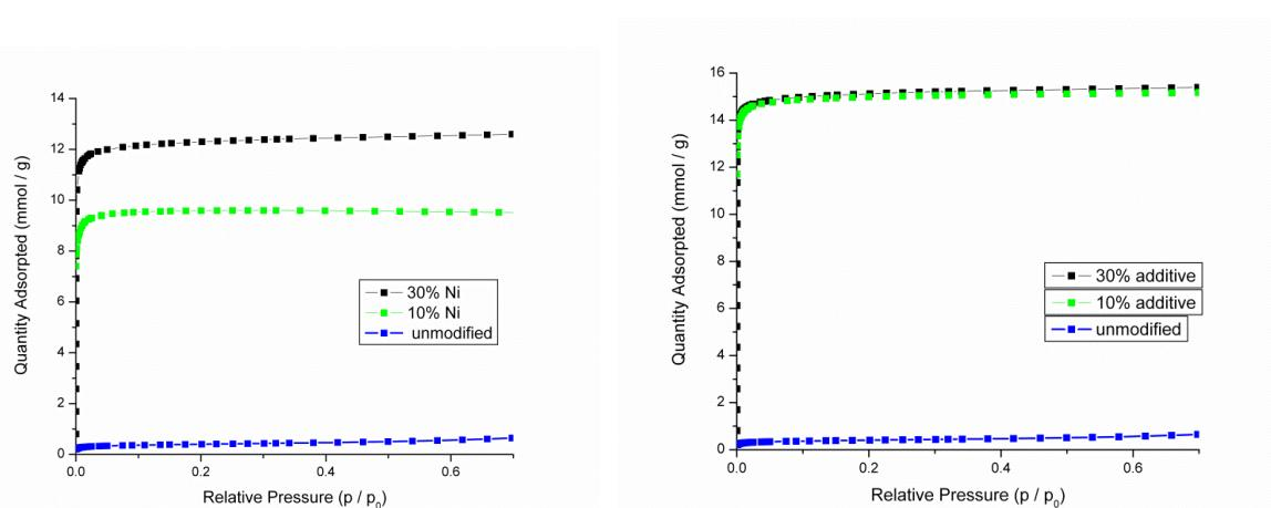
Figure S5.1 (Left) N<sub>2</sub> adsorption (77K) of CPO-27(Mg) and material modified with 10% and 30% of nickel acetate and 10% *cpmp* after samples were activated at 373K followed by 523K. (Right) N<sub>2</sub> adsorption (77K) of CPO-27(Mg) and material modified with 10% and 30% of nickel acetate and 10% *cpmp* where samples have been activated for a second time at 373K followed by 523K.
