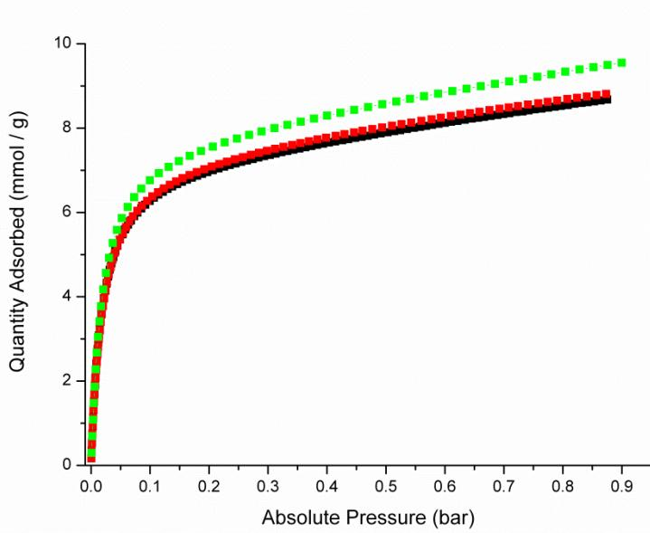
Figure S9.2: Repeated CO<sub>2</sub> adsorption (298 K) of CPO-27(Mg) modified with 10% nickel acetate and 10% *cb/m*. Samples were obtained as described in experimental part from 3 different syntheses and have been activated at 373K followed by 553 K before measurement.
