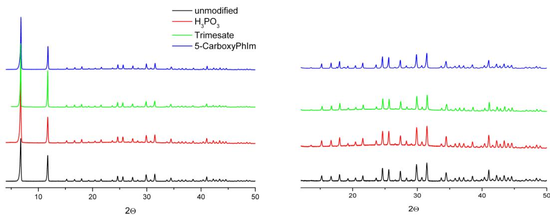
Figure S4.2 PXRD of unmodified CPO-27(Mg) and also CPO-27(Mg) modified with 10% nickel acetate and different acids.
