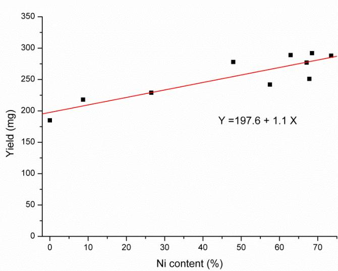
Figure S6.1 Yield (mg) vs. Ni content (%) observed by EDX analysis of nickel and *cpmp* modified CPO-27(Mg) materials, all with the same starting amounts and conditions in the first synthesis step (see paper for details).
