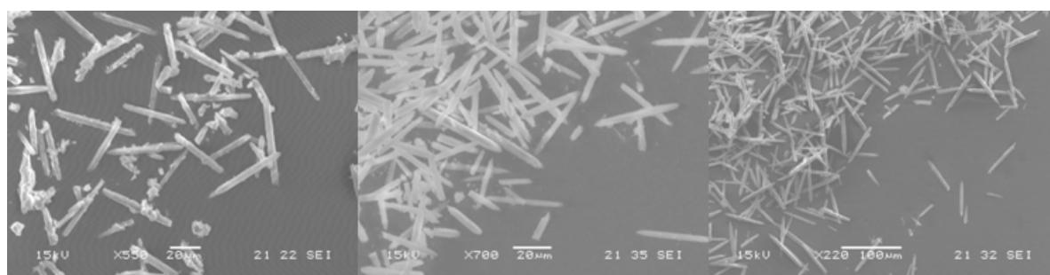
Figure S8.1 SEM images of CPO-27(Mg) modified with 70%  $\text{Ni}^{2+}$  and 10% *cpmp* recorded after different second step reaction times. 1 hour (left), 8 hours (middle), 3 days(right).
