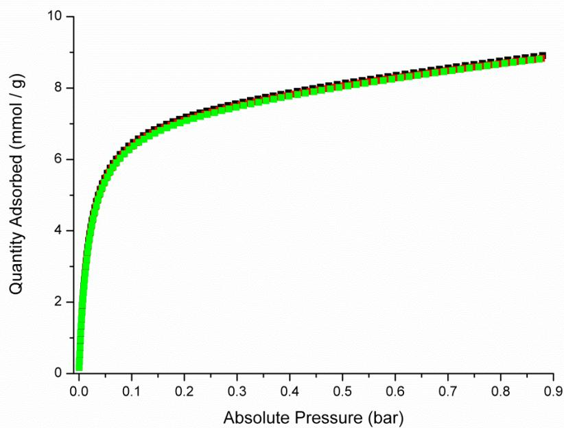
Figure S9.1: Repeated CO<sub>2</sub> adsorption (298 K) of CPO-27(Mg) modified with 10% nickel acetate and 10% *cb/m*. The same batch has been activated at 373 K followed by 553 K and measured 3 times. First (green), second (red), third (black).
